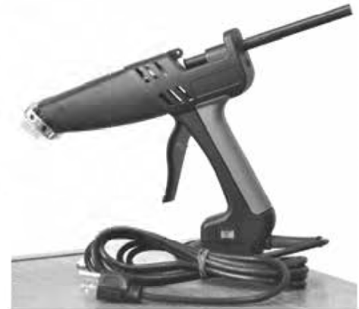
Figure 29. Enviro Liner Welding Gun
