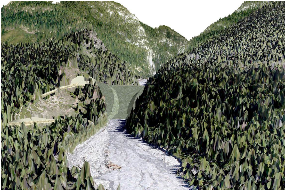
Revised vegetated spillway design – no water impoundment
