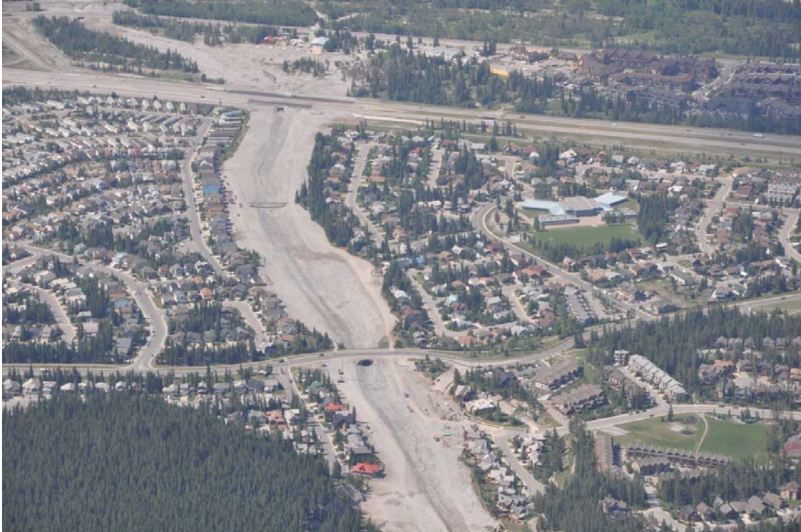
Photo A-39. Aerial view of reconstructed Cougar Creek looking downstream from about the fan apex. BGC photograph of July 23, 2013.
