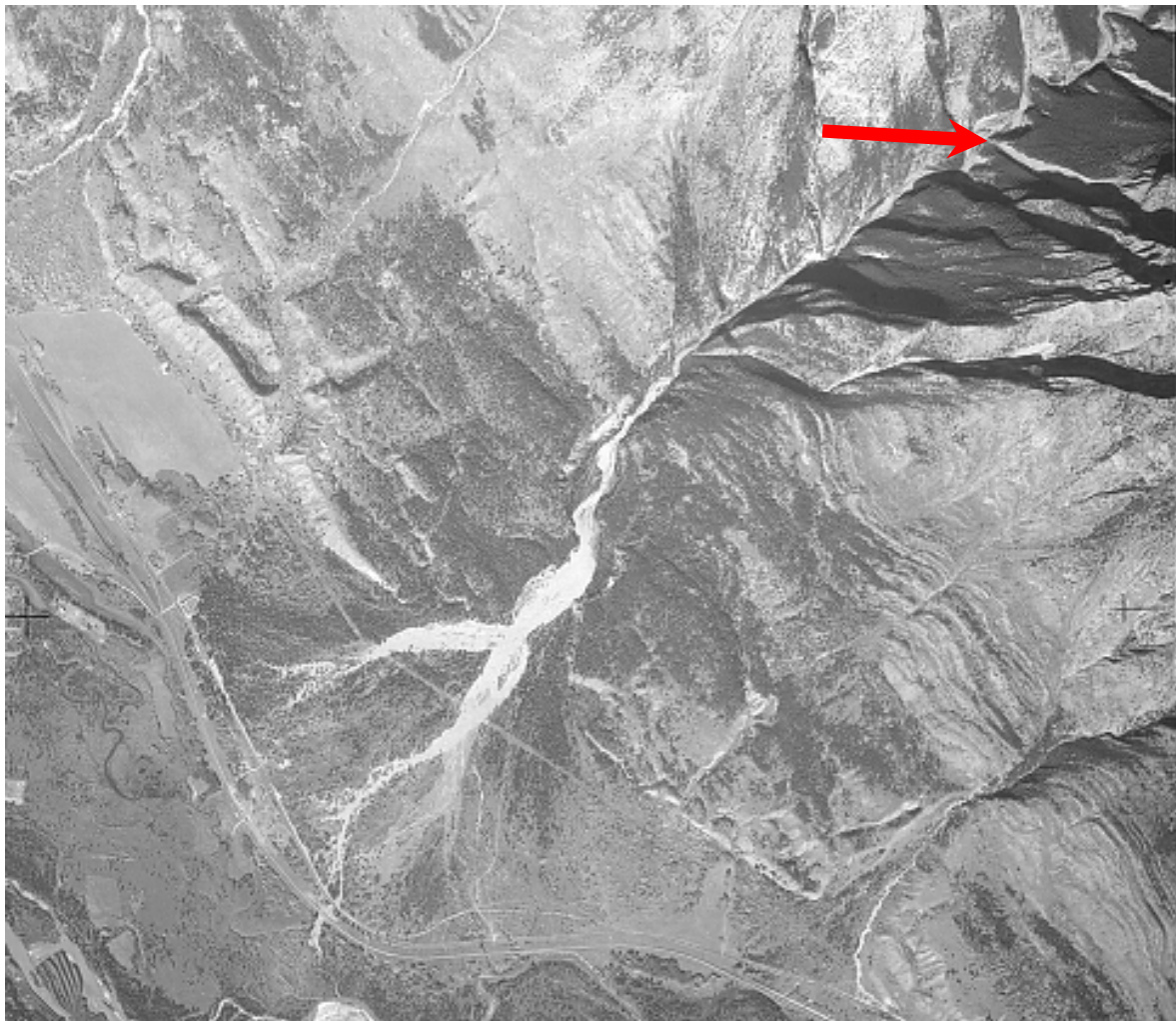
Figure 7-2. 1950 air photograph of the lower reaches of Cougar Creek and the fan. The red arrow indicates a relatively fresh debris avalanche that may have dammed Cougar Creek leading to a landslide dam outbreak flood.
