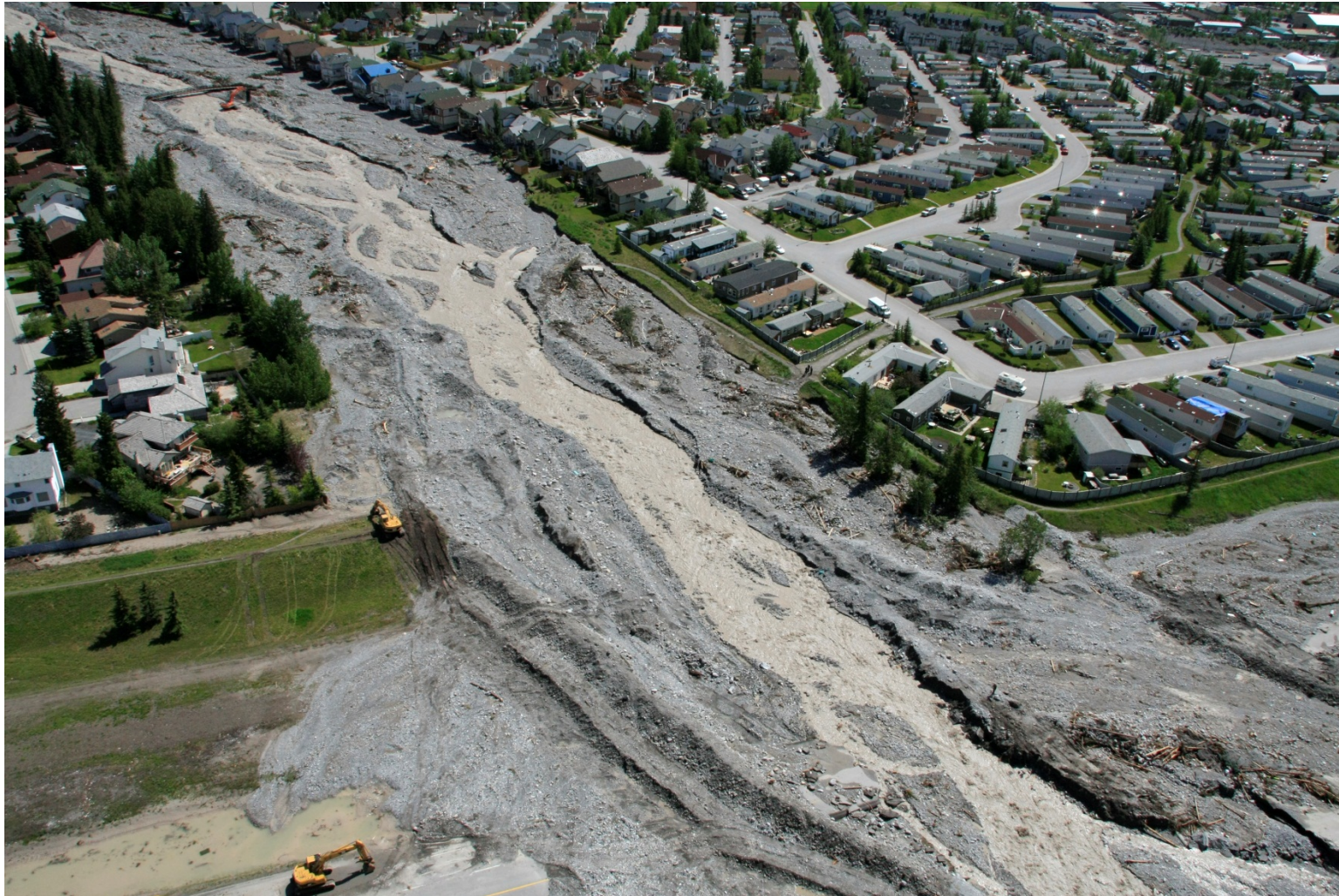
Photo A-28. Aerial view of restoration efforts along Cougar Creek at Highway 1 following the 2013 debris flood. Photograph courtesy of the Town of Canmore.
