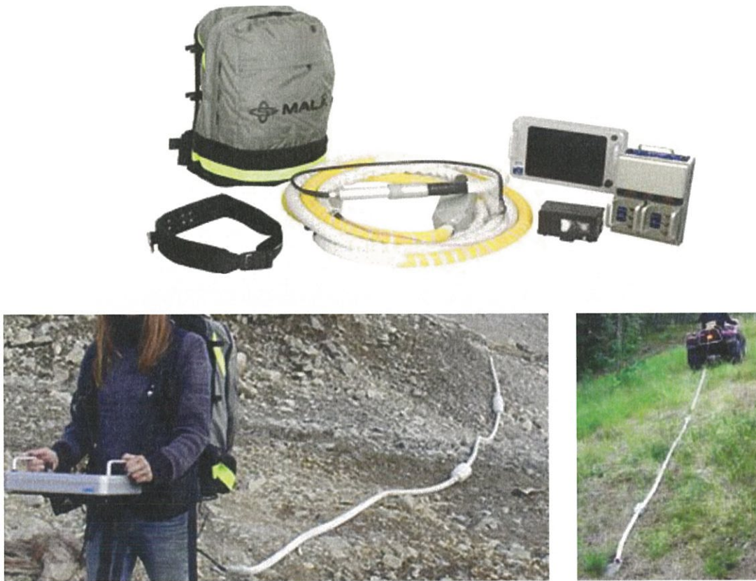
Figure 2-3 Top – MALA 100 MHz RTA (Rough Terrain Antenna) and survey components. Bottom Left: Operator manually dragging a rough terrain antenna. Bottom Right: ATV dragging a rough terrain antenna.
