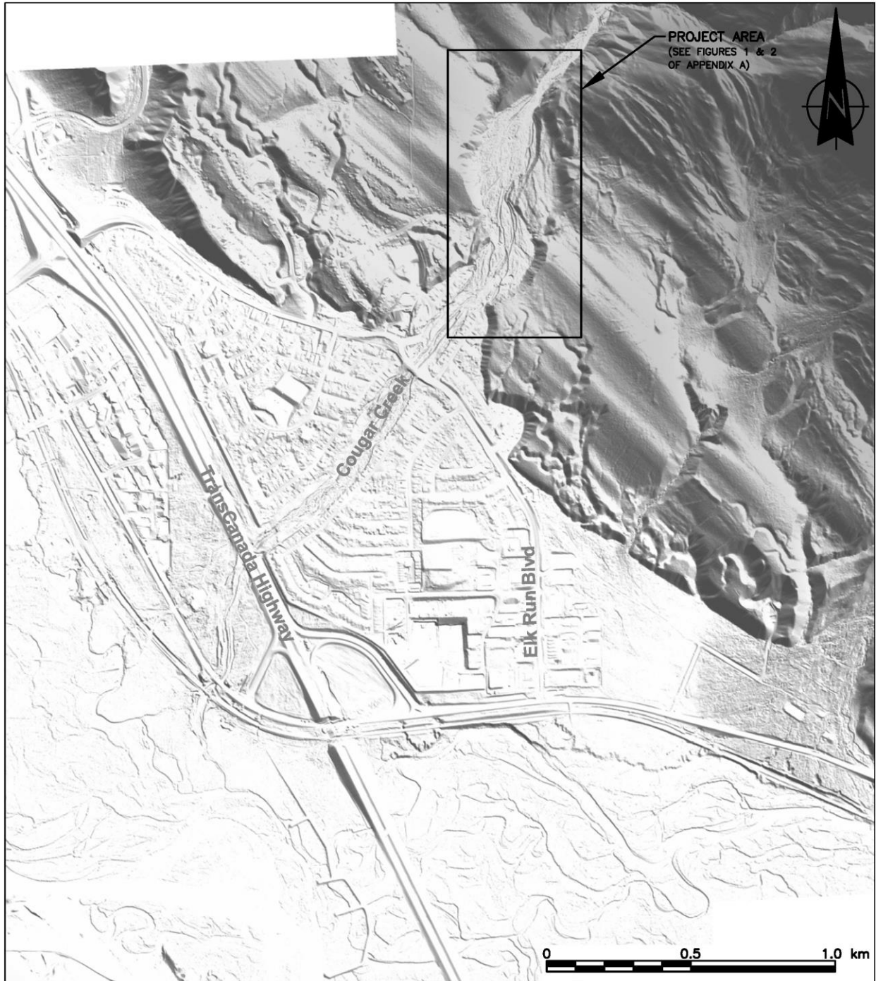
Illustration 3. 2013 post-flood LiDAR imagery provided for the Town of Canmore. Note erosion of the glacial deposits by Cougar Creek (boxed area)
