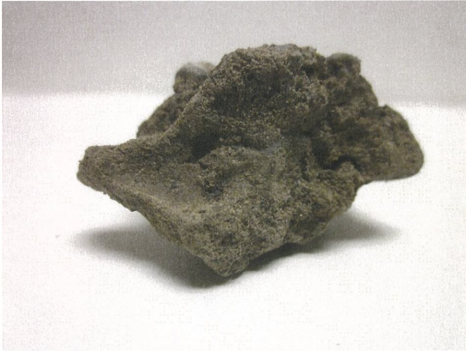
Photo 3: Crumb Test Sample 2 (Valley Wall) – Before Immersion
