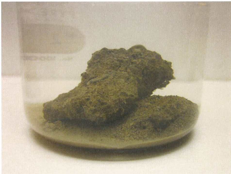
Photo 4: Crumb Test Sample 2 (Valley Wall) – After 24 hrs Immersion
