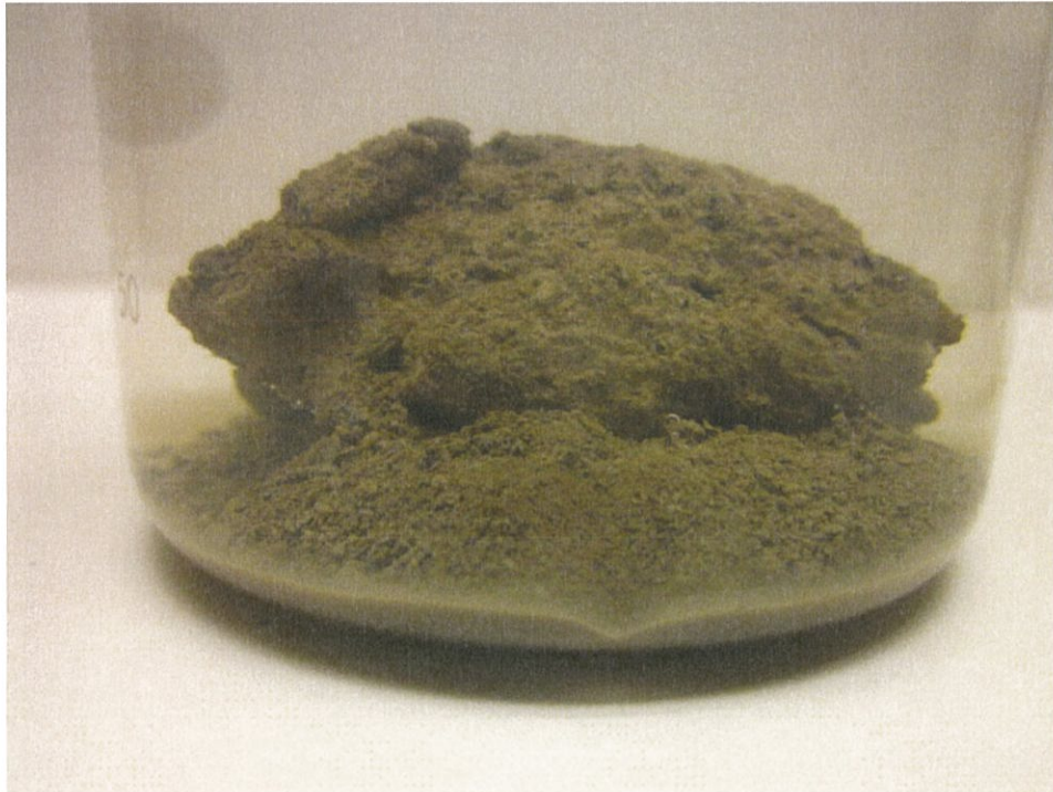
Photo 2: Crumb Test Sample 1 (Valley Wall) – After 24 hrs Immersion
