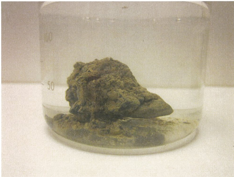
Photo 6: Crumb Test Sample 3 (TP14-06) – After 24 hrs Immersion
