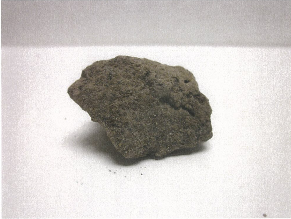
Photo 1: Crumb Test Sample 1 (Valley Wall) – Before Immersion
