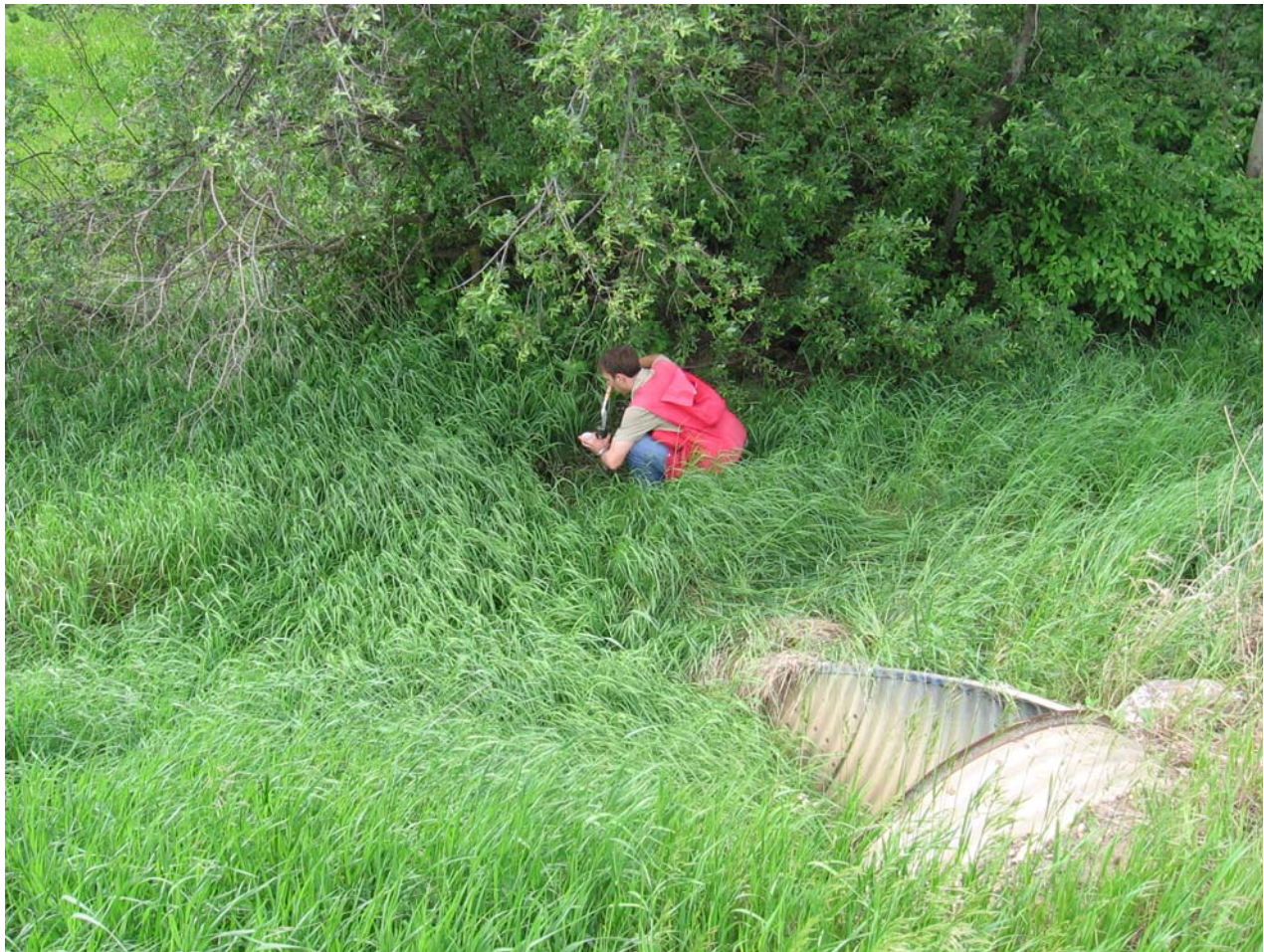
Photo III-3: Sediment Sampling Location SED3 Looking South (June 14, 2006). Conveyance under Township Road 560 is via a 1,219 mm Corrugated Steel Culvert. No Free Water, only Sediment was Sampled at this Location
