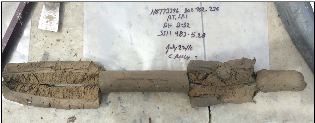
Figure 22. Sample of Glaciolacustrine Clay and Silt Recovered from 4.8 to 5.3 m depth in D32
