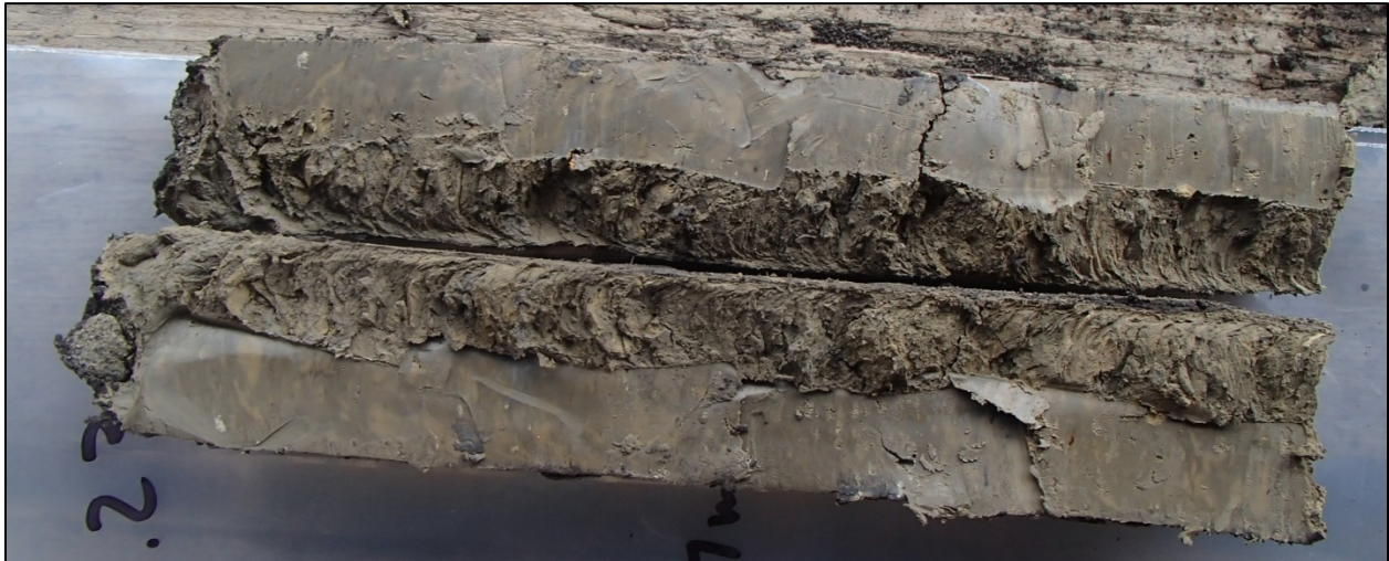
Figure 21. Sample of Glaciolacustrine Clay and Silt Recovered from 2.3 to 2.7 m depth in D20
