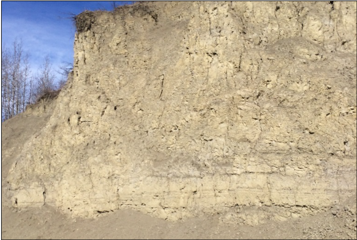
Figure 26. Stratified Layer observed near the base of the Upper Brown Glacial Till in OC14
