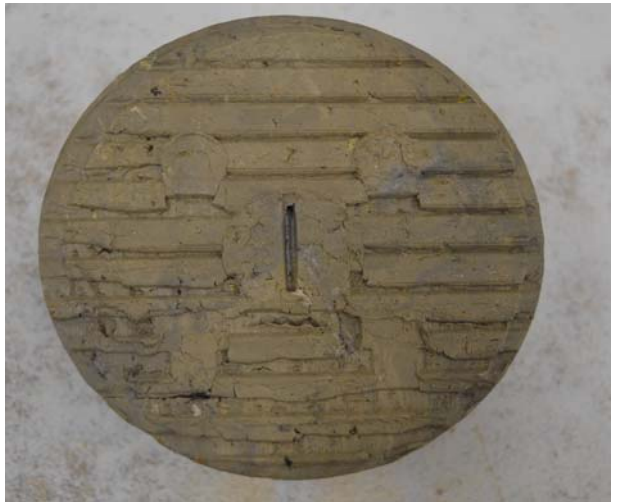
Bottom of sample showing groove indentations from bottom platten with raised fins. Picture also shows slip along bottom interface
