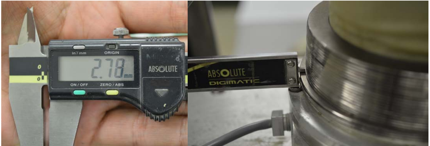
Ring alignment after completion of the test. Porous stones are at level with the slipped ring.
