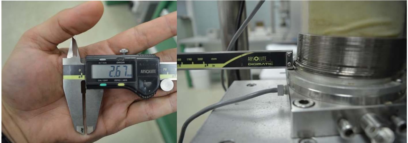
Ring alignment after completion of the test. Porous stones are at level with the slipped ring.
