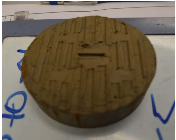
Bottom of sample showing groove indentations from bottom platten with raised fines. Picture also shows slip along bottom interface
