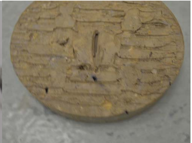
Bottom of sample showing groove indentations from bottom platten with raised fines. Picture also shows slip along bottom interface
