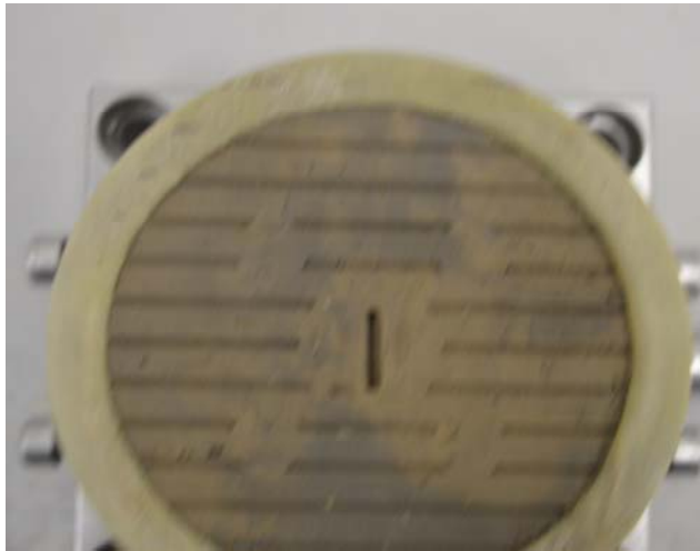
Top of sample showing groove indentations from top platten with raised fins
