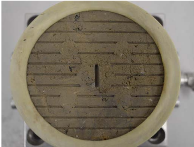
Top of sample showing groove indentations from top platten with raised fins
