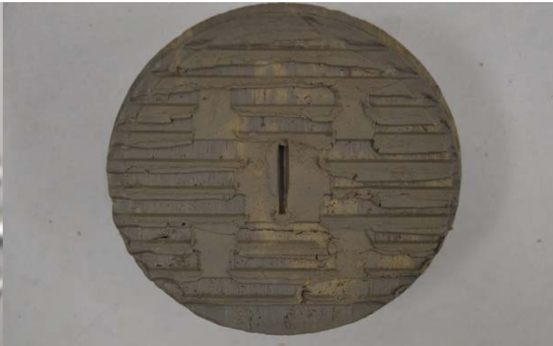
Bottom of sample showing groove indentations from bottom platten with raised fins. Picture also shows slip along bottom interface
