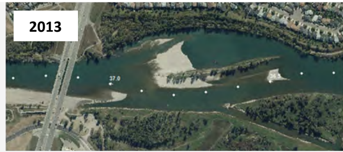
Bow River avulsion through a former gravel pit at Carburn Park during the 2013 flood
