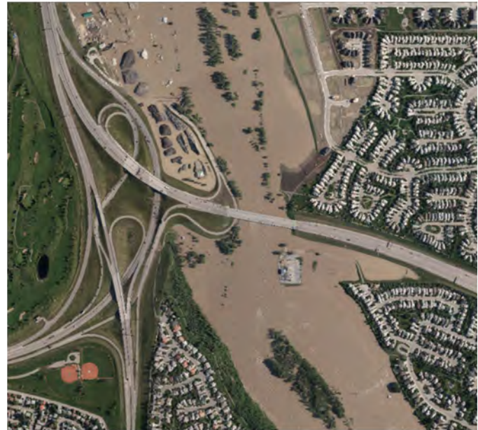
Bow River flow constriction at Ivor Strong Bridge during the 2013 flood
