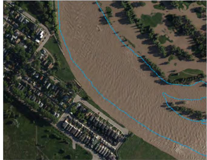
Bank erosion in Inglewood during the 2013 flood. The blue line shows the pre-flood bank.
