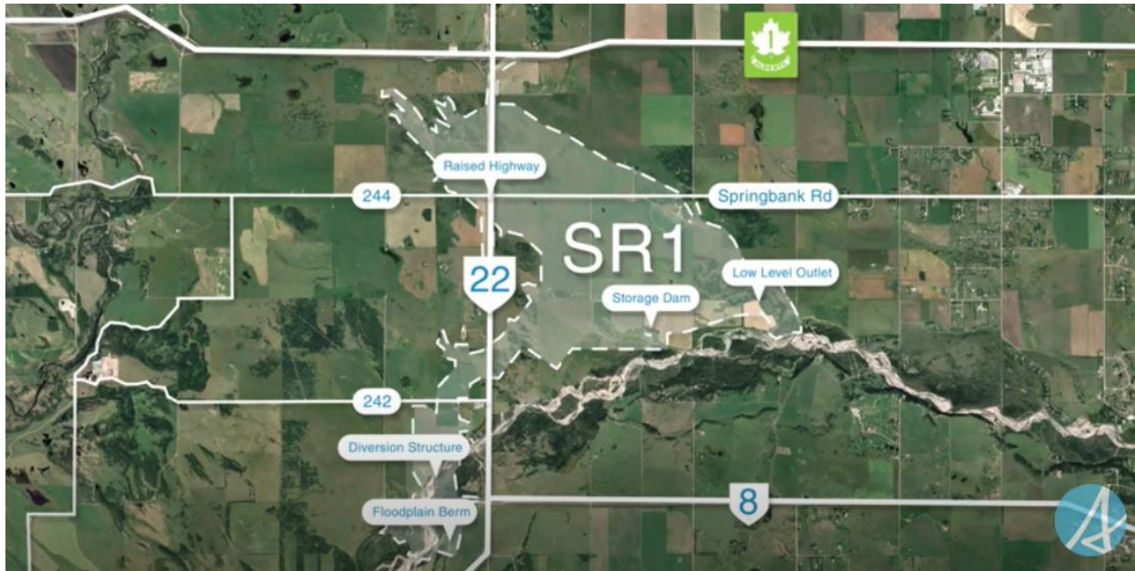
Figure 1. Springbank Off-stream Storage Reservoir Project (SR1) component locations (Source: Government of Alberta)
