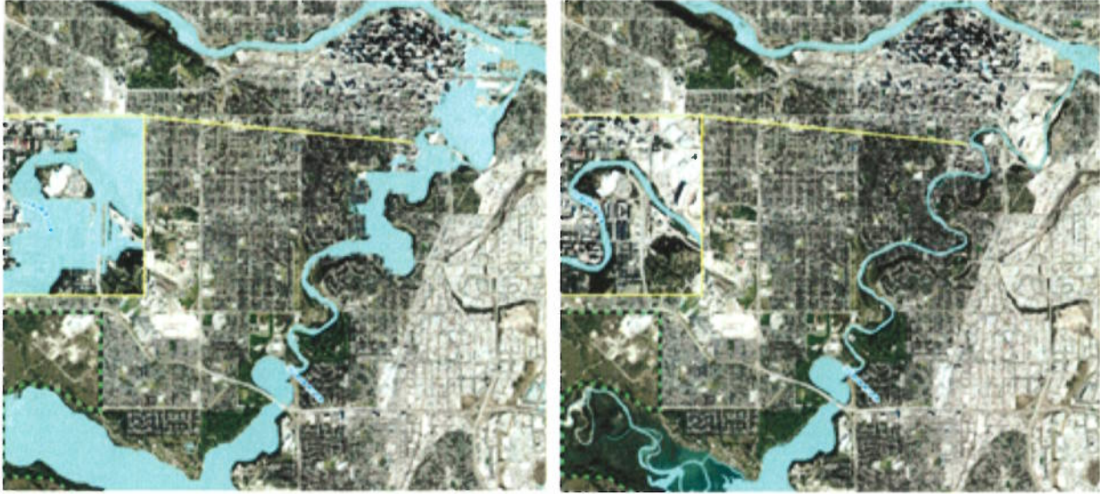
Figure 3 – The 2013 Elbow River flood extents (left), and what the flooding would have looked like if the Springbank Project had been in place (right).
