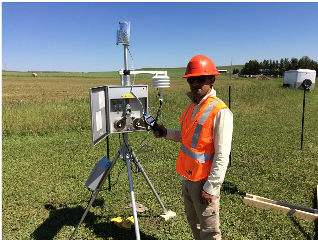
Photo 3D-3 Calibration of EBAM Monitor Prior to Background TSP Monitoring at Parcel 56. August 2, 2016 (Looking Northeast).
