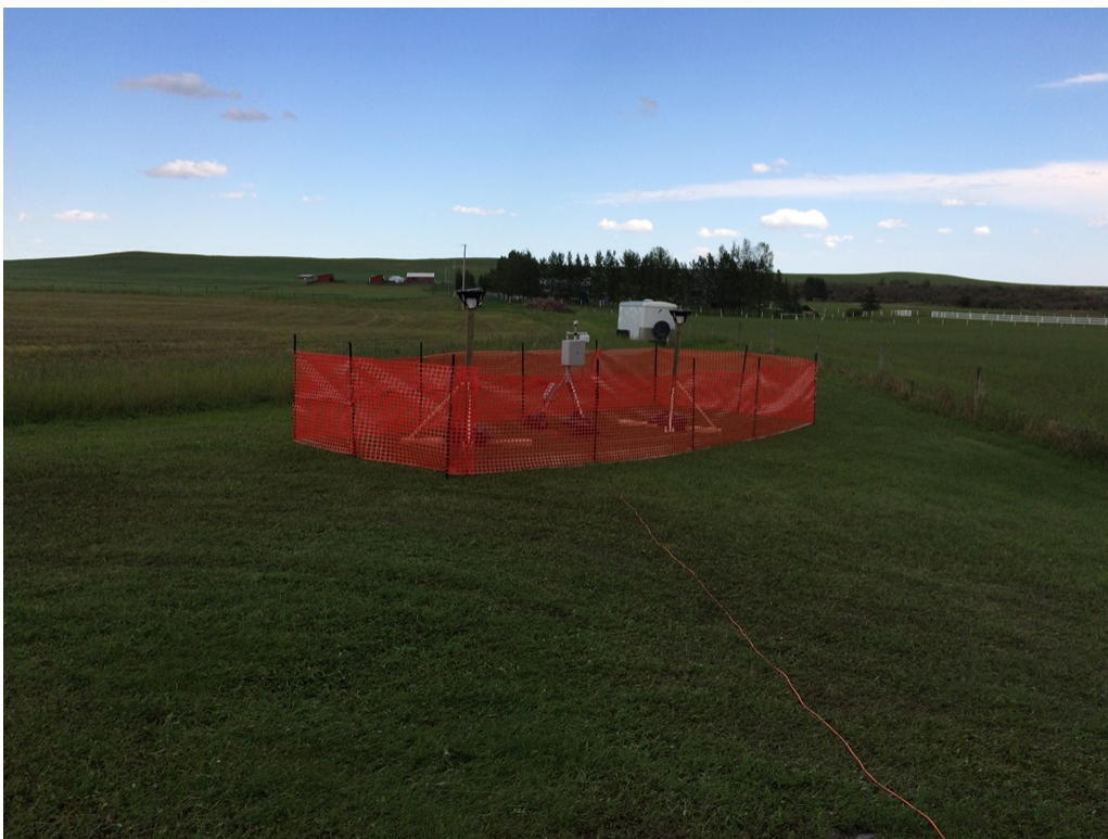
Parcel 56 – View East Toward E-BAM Particulate Monitor and dustfall collectors (August 2, 2016)
