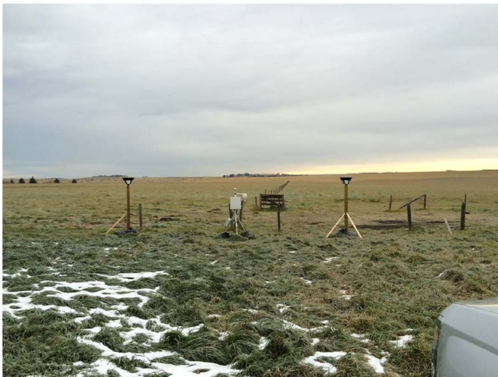
Photo 3D-2 EBAM Monitor (Centre) and Dustfall Collectors (Left and Right) at Parcel 58 on October 13, 2016 (Looking North).
