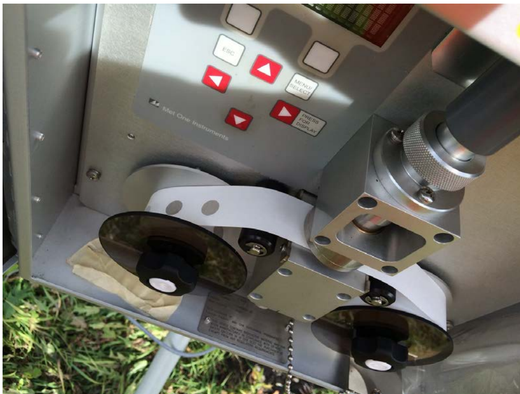
Photo 3D-4 Particulate Matter (PM) Deposited on EBAM Filter Tape (Grey Circles). October 13, 2016
