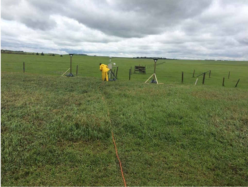
Parcel 58 – View North Toward E-BAM Particulate Monitor and dustfall collectors (August 3, 2016)
