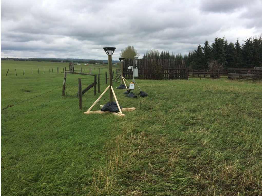
Parcel 58 – View East Toward E-BAM Particulate Monitor and dustfall collectors (August 3, 2016)
