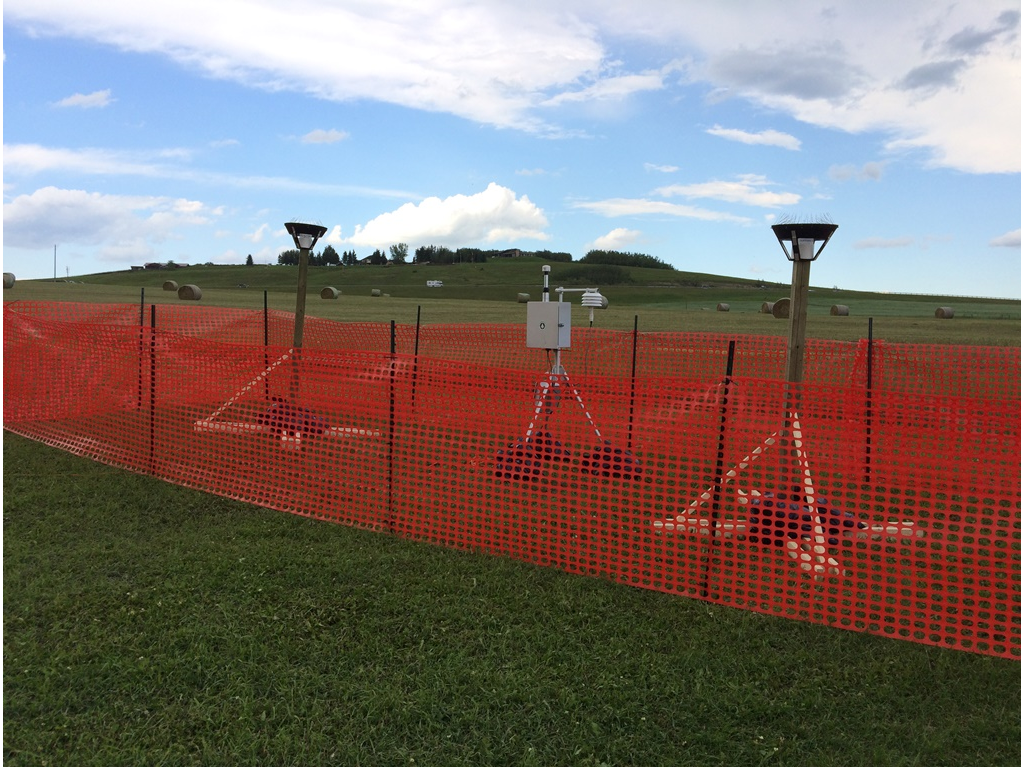
Parcel 56 – View North Toward E-BAM Particulate Monitor and dustfall collectors (August 2, 2016)
