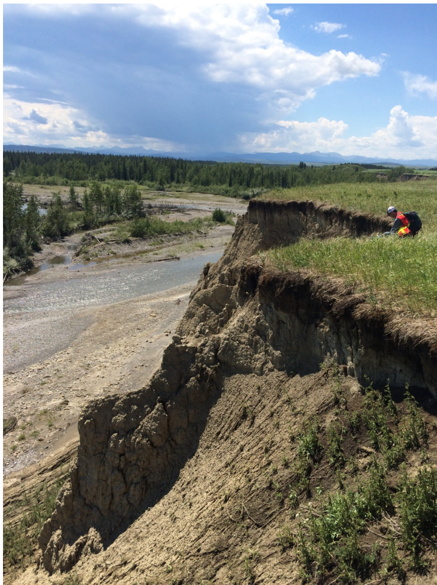
Photo 2-8 Debris Avalanche Along the Elbow River Scarps Exposing Glaciolacustrine Silt and Clay Overlying Consolidated Clay Till.
