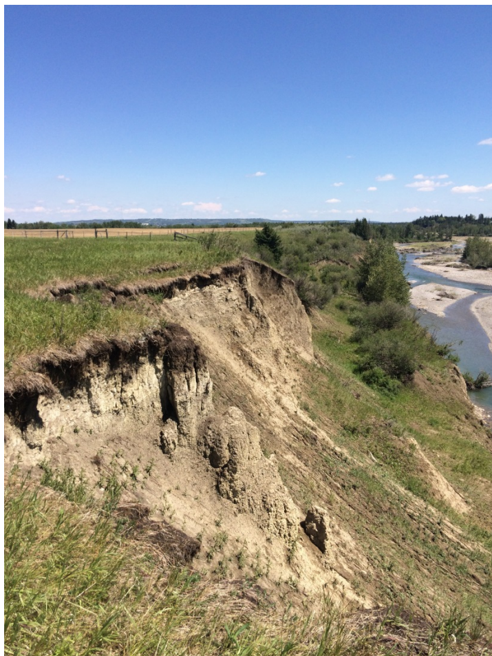
Photo 2-5 Field photo showing colluvium deposits, derived from glaciolacustrine material on over-steepened scarps adjacent to the Elbow River
