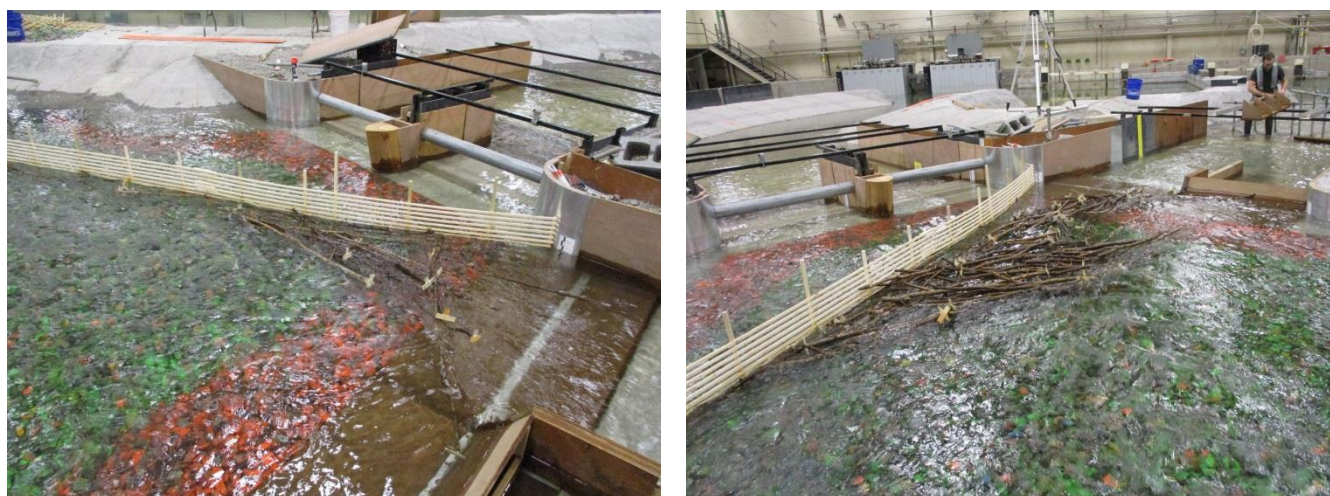
Figure 174. Debris being caught at the downstream end of the barrier and bridging across the LHS of the service spillway to start a jam (left), and the jam building through the testing program (right).
