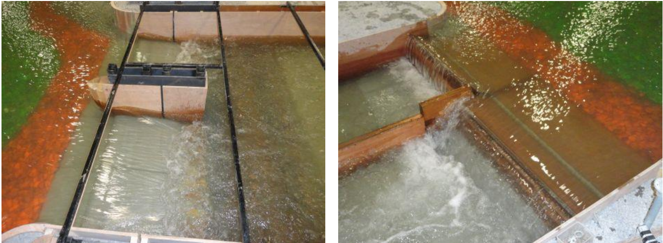
Figure 123. Flow conditions at the structure during the 760 m 3 /s event with the Obermeyer gates set to 1213.4m (LHS) and 1215m (RHS). Left - facing southwest at the diversion, right - facing southeast at the service spillway.
