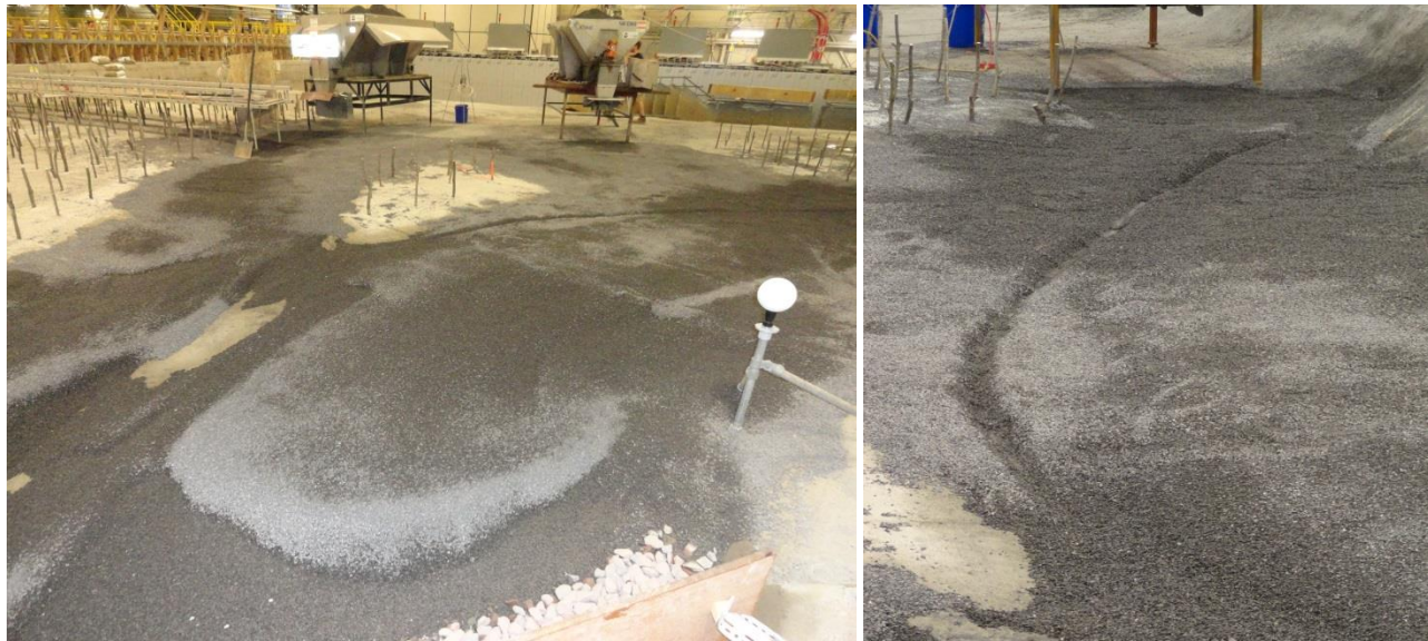
Figure 114. Initial upstream mobile bed conditions prior to the 1240 m 3 /s flow condition.
