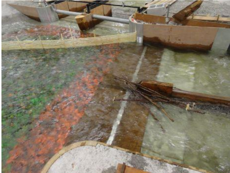
Figure 178. Debris remaining caught on the dividing pier after lowering the Obermeyer gates after all of the gate operations of the 500\text{m}^3/\text{s} Case B flow condition.
