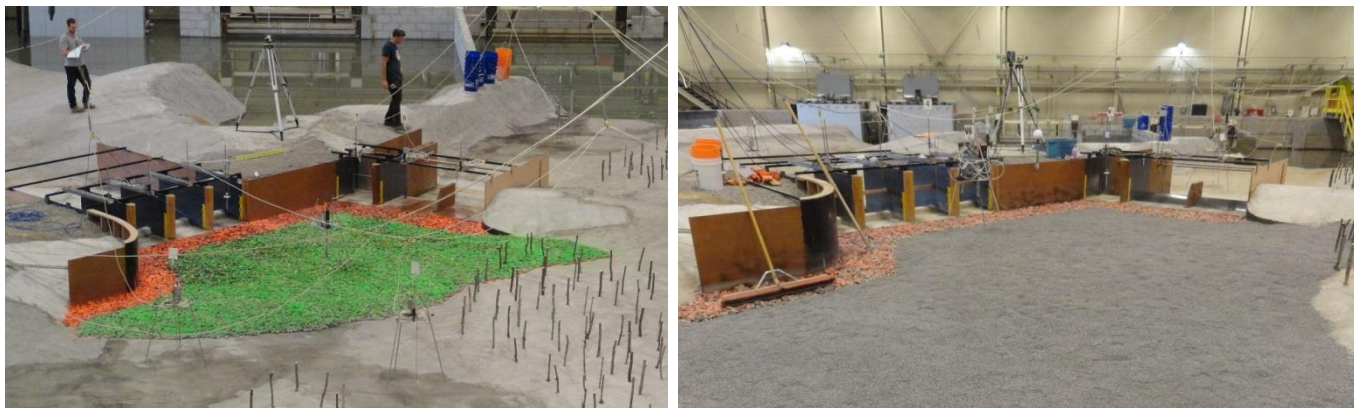
Figure 34. Left – mobile bed area of the model was filled with 210kg (green) riprap stone during clear water or debris tests. Right – model river sediments placed in the mobile bed area.
