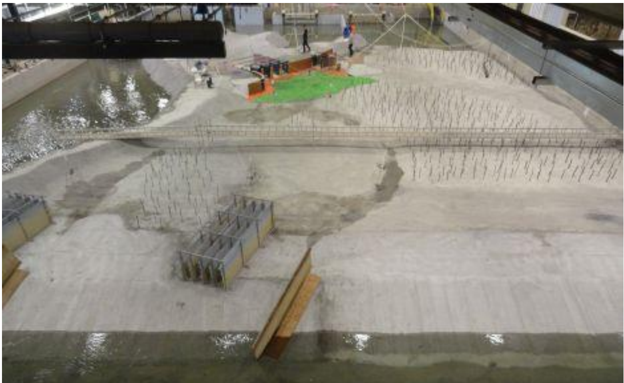
Figure 23. Photograph of the physical model after construction – looking downstream.
