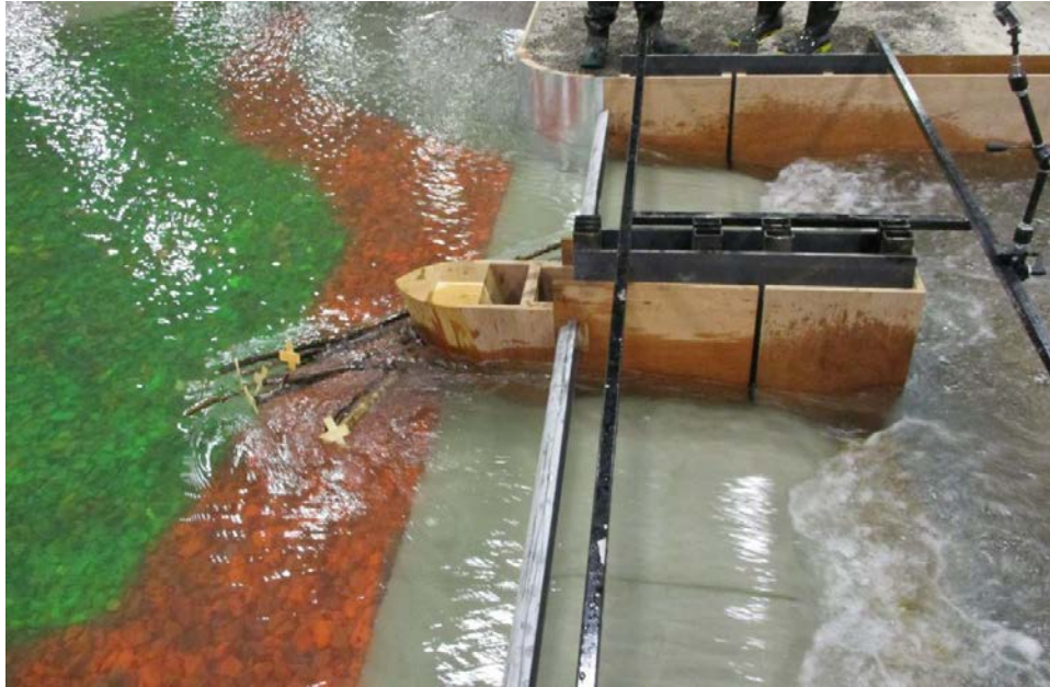
Figure 130. Debris caught on Pier Nose 3.
