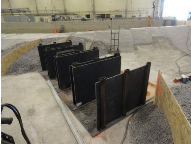
Figure 38. Left: diversion inlet pier struts and base plates installed in the basin. Right: precision milled hardwood pier noses after manufacture.
