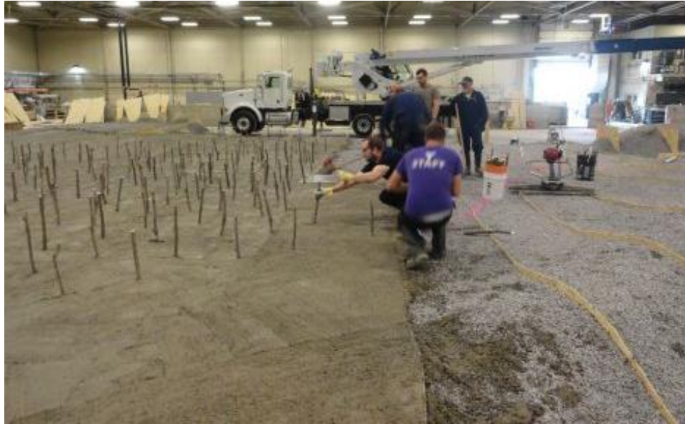
Figure 31. The concrete was broom finished to roughen the surface, and model trees were inserted into the wet concrete to model forested regions of the floodplain.
