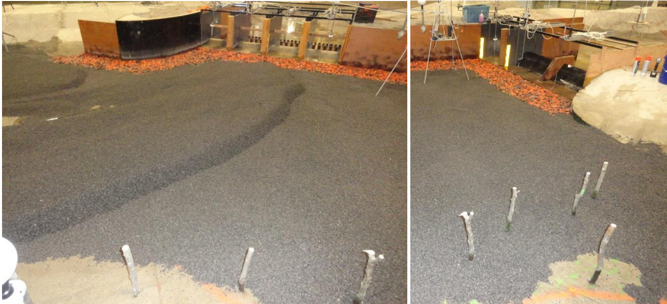
Figure 105. Deposition and erosion in the forebay area after 320 m 3 /s flow condition.
