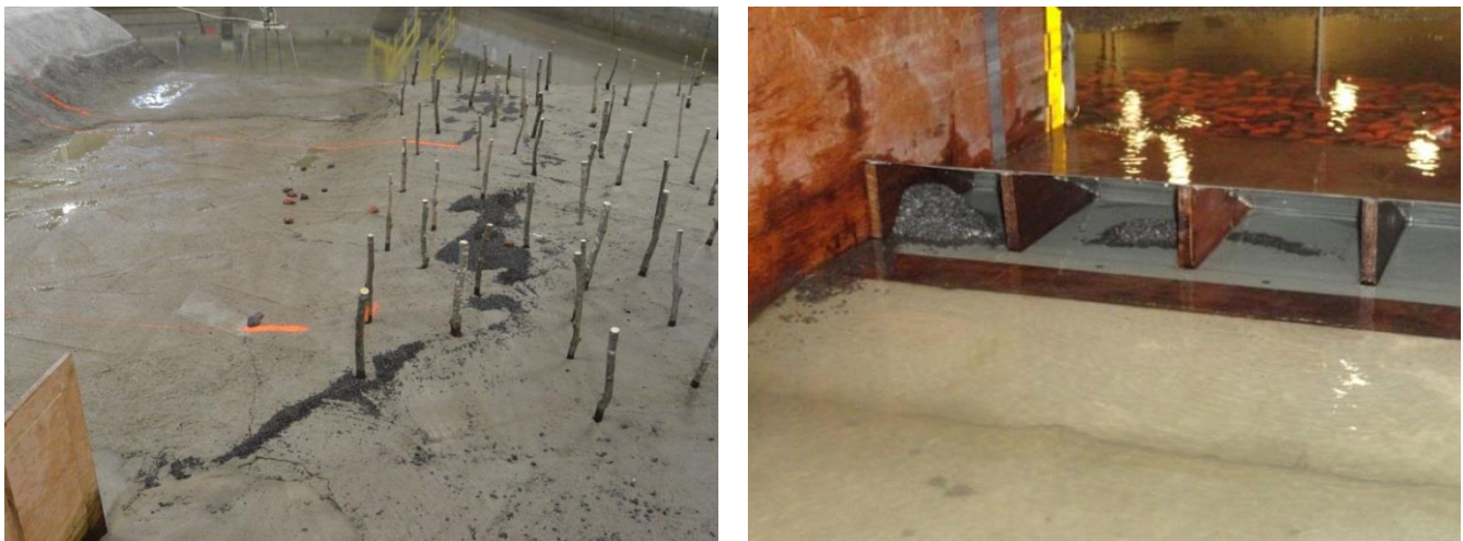
Figure 118. Sediment deposited downstream of the service spillway structure along the RHS of the channel (left) and underneath the Obermeyer gates (right).
