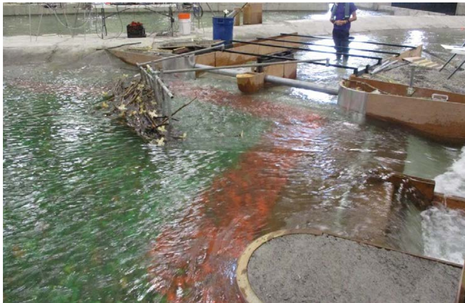
Figure 149. Debris collected on barrier C at the start of the tests.
