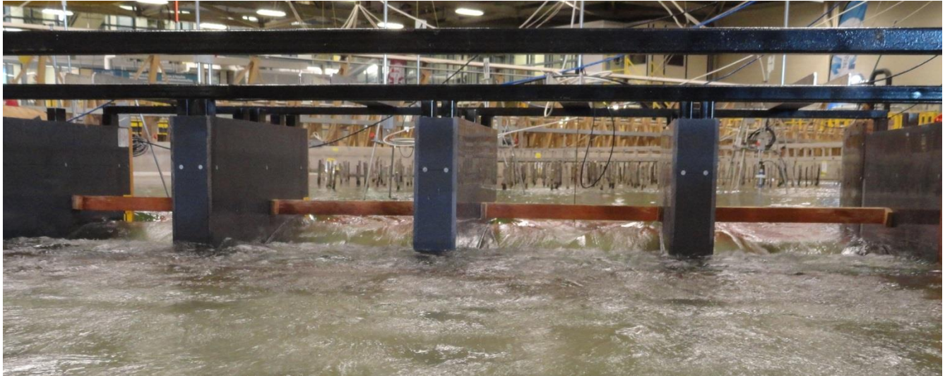
Figure 90. Turbulent flows downstream of diversion inlet gates.
