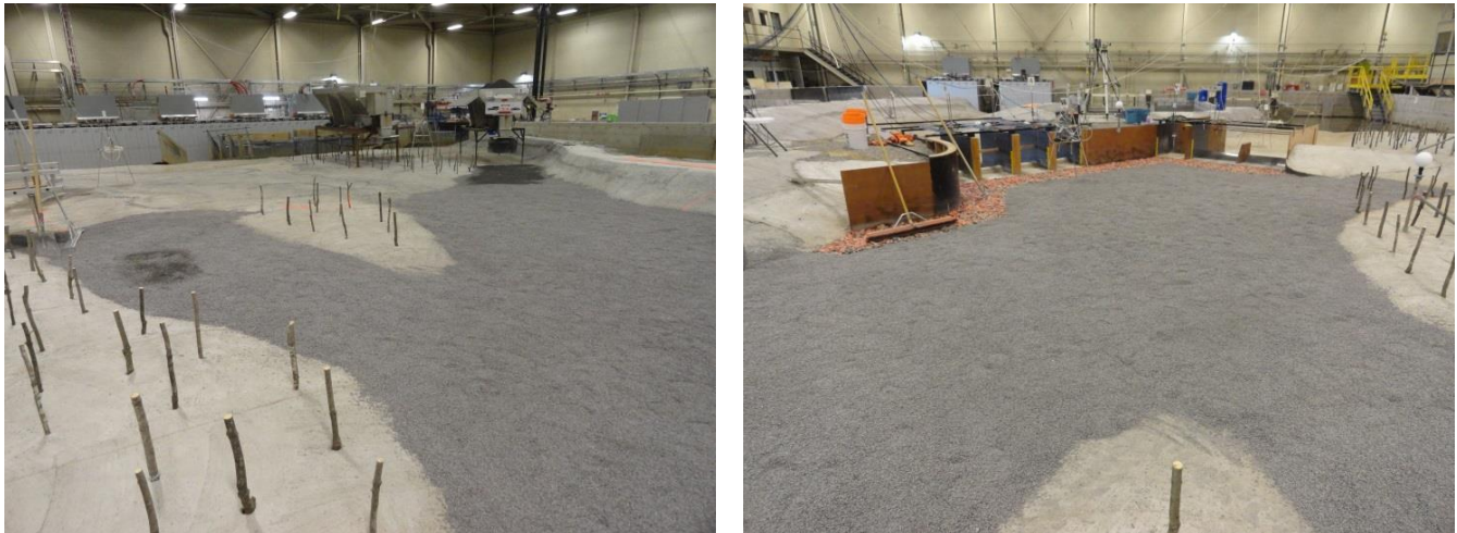
Figure 73. Preloaded sediment in the main channel and secondary channel (left) and in front of the structures (right).
