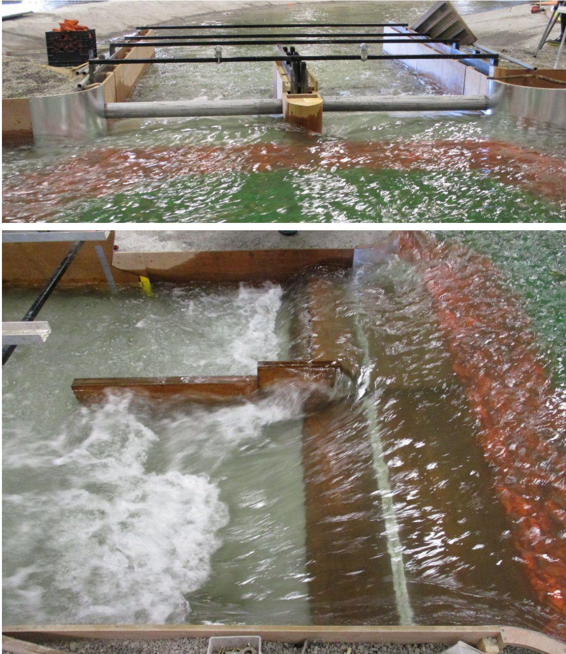
Figure 144. Flow conditions at the structure during the 1240 m 3 /s event. Top – facing downstream at the diversion, bottom - facing southeast at the service spillway.
