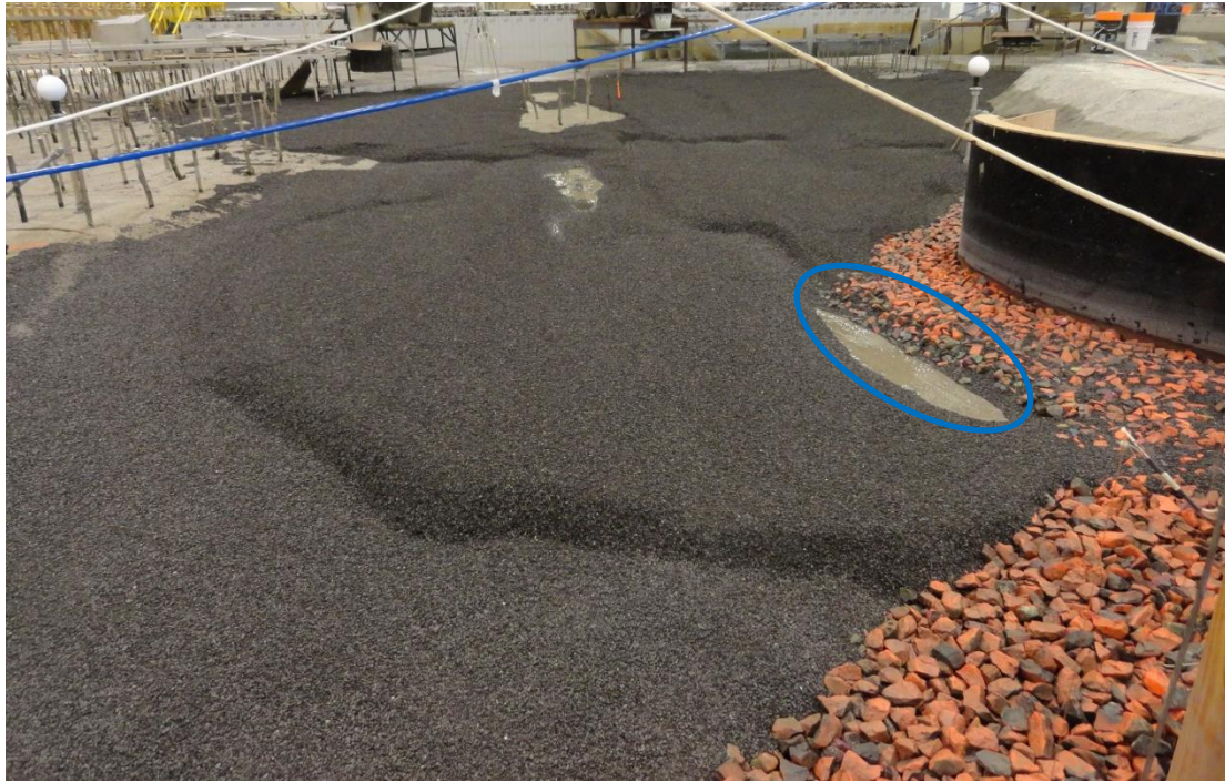
Figure 115. General view of the mobile bed in the forebay area after the 1240 m 3 /s flow condition (new scour hole highlighted).
