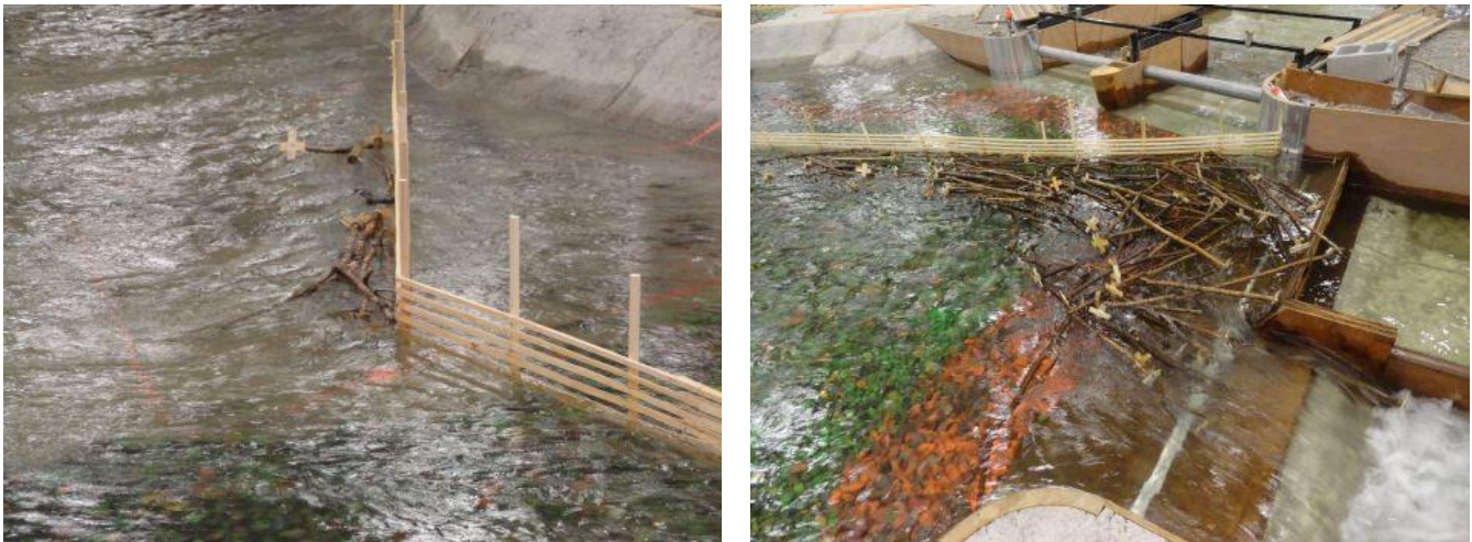
Figure 177. Debris caught on the upstream end of the barrier (leg AB) at the end of the Case B tests (left) and at the downstream end of the barrier (leg BC) in front of the raised LHS Obermeyer gate (right).
