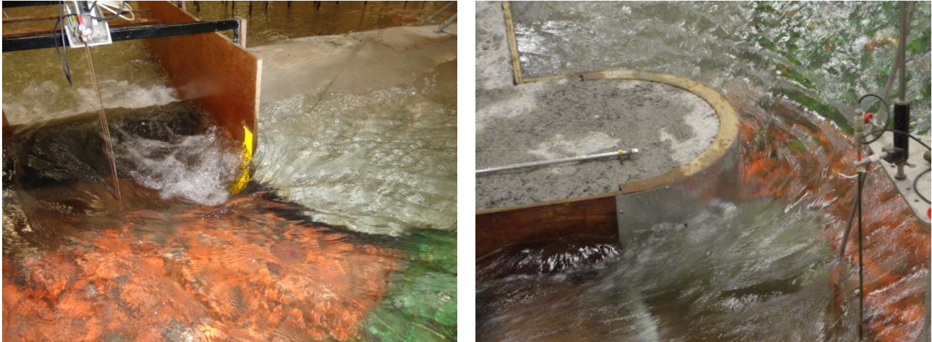
Figure 163. Wakes generated by the retaining wall on the RHS of the service spillway – left: straight wall of the initial design, right – circular design for TSD-H.
