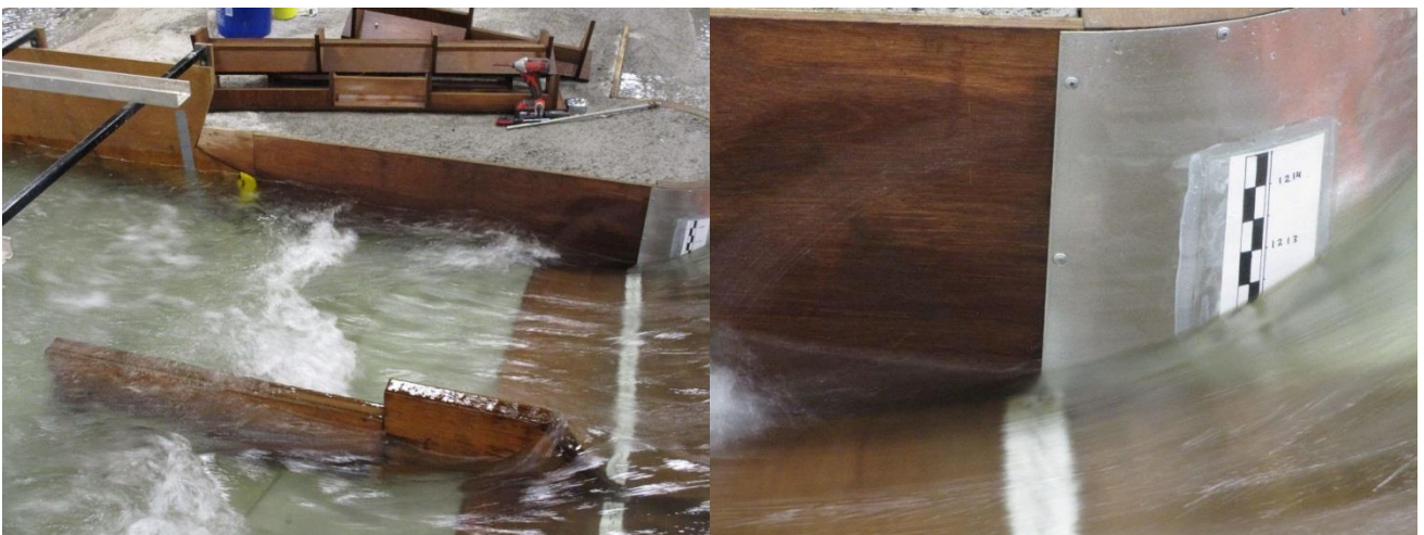
Figure 161. Flow through the diversion inlet structure (left) and service spillway (right) during the 760 m 3 /s case (b) flood condition.
