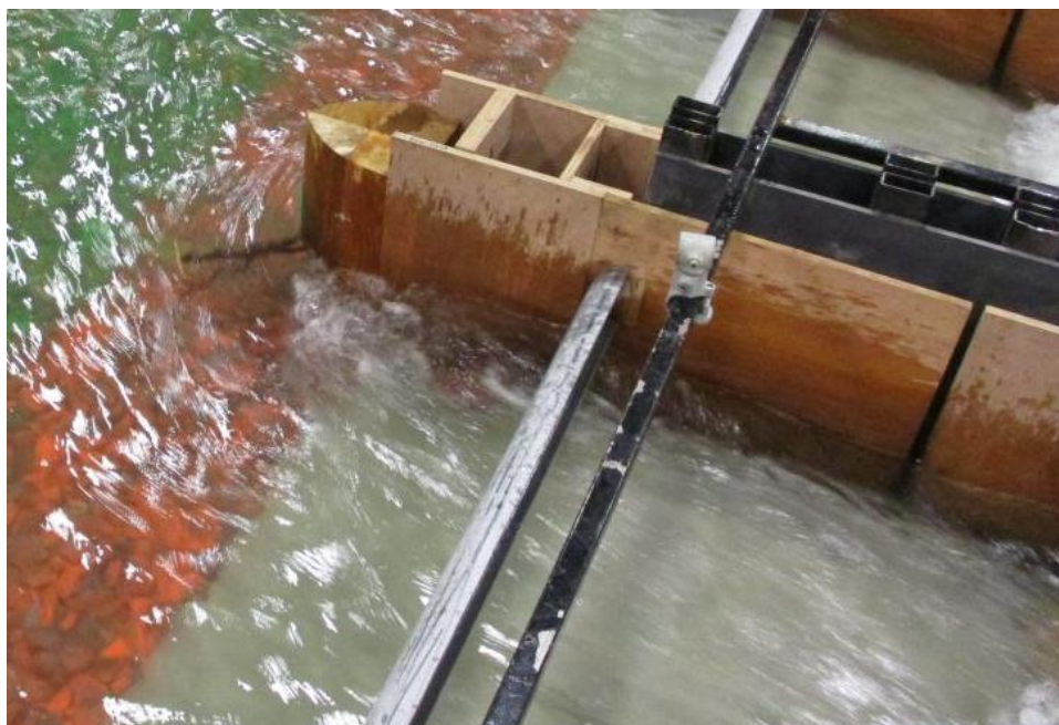
Figure 147. Debris caught on Pier Nose 2.
