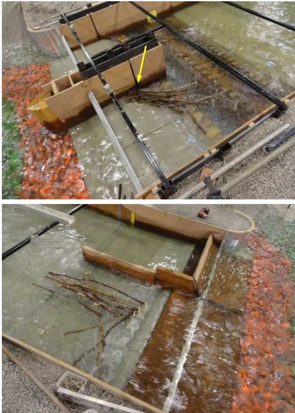
Figure 152. Debris caught in the structures during the 320\text{m}^3/\text{s} flow condition with pier nose 2.
