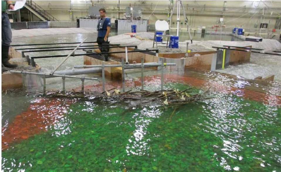
Figure 136. Debris caught on Debris Barrier B.
