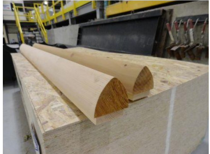
Figure 38. Left: diversion inlet pier struts and base plates installed in the basin. Right: precision milled hardwood pier noses after manufacture.
