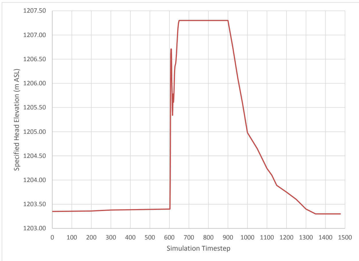
Figure 5-3 Example Hydrograph Used for Time Varying Specified Head Boundary Conditions in Diversion Channel
