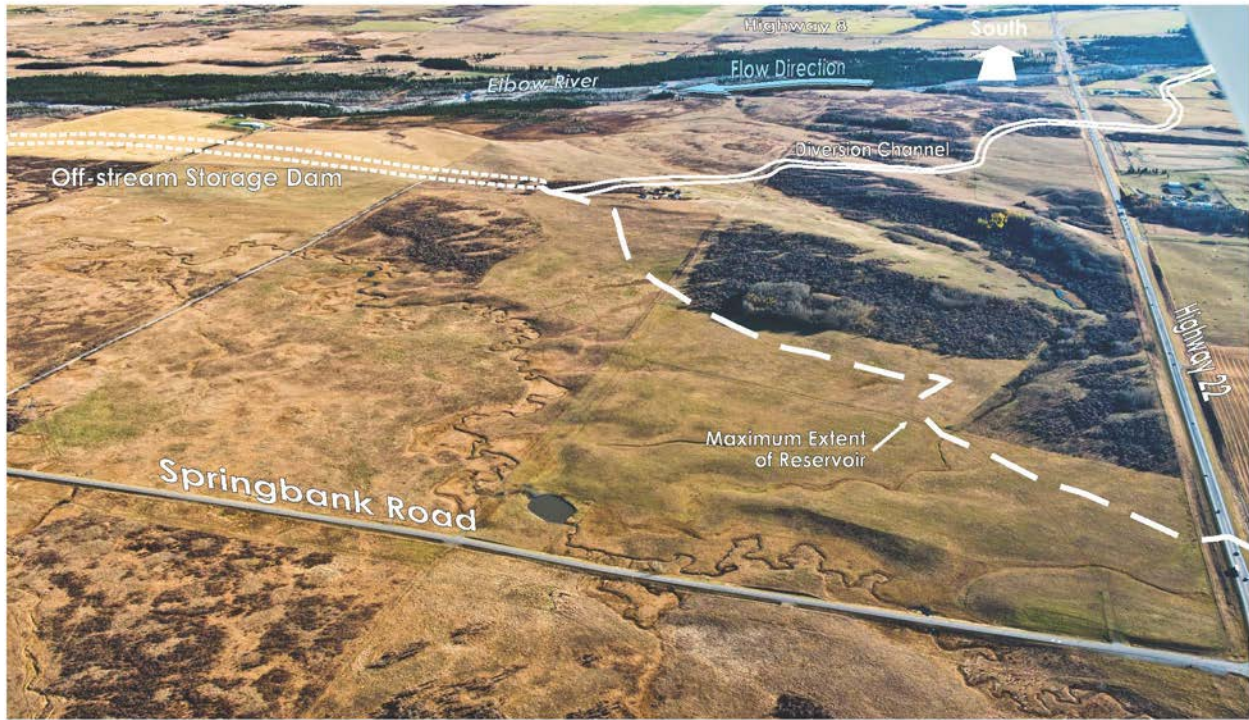
Figure 3-2 Looking South towards Off-stream Storage Reservoir, Off-stream Storage Dam and Diversion Channel Locations
