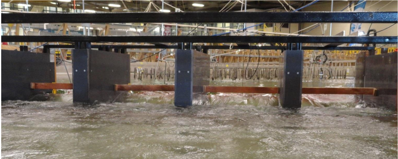
Figure 90. Turbulent flows downstream of diversion inlet gates.
