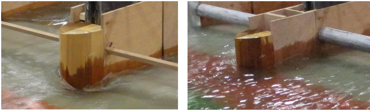
Figure 125. Flat breast wall on Pier Nose 1 (left) and curved breast wall (right) used for all future debris tests (Pier Nose 2 shown).
