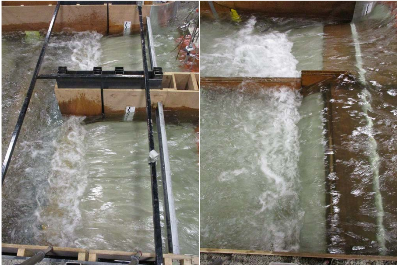
Figure 164. Flow through the diversion inlet structure (left) and service spillway (right) during the 1240 \text{ m}^3/\text{s} case (b) flood condition.
