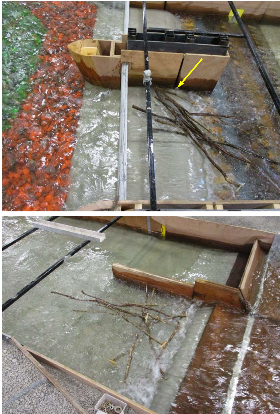
Figure 153. Debris caught in the structures during the 320\text{m}^3/\text{s} flow condition with pier nose 3.
