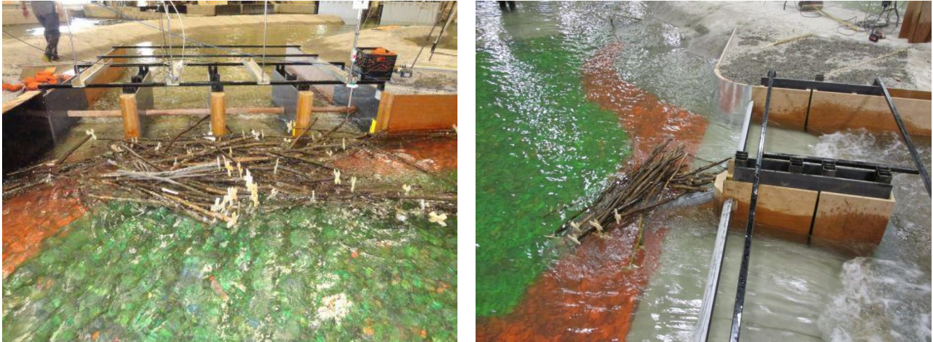
Figure 70. Woody debris interacting with the structures: left – the original diversion, right – the revised diversion inlet with pier nose 4.
