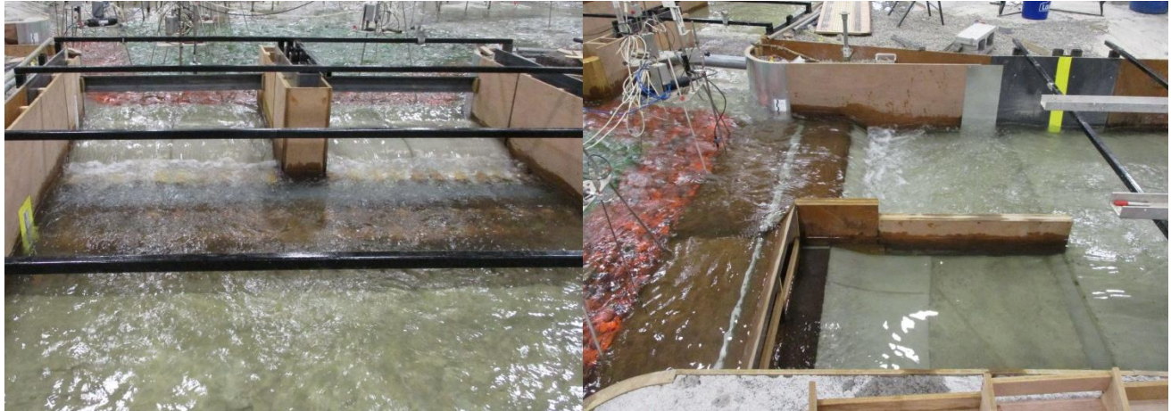
Figure 157. Flow through the diversion inlet structure (left) and service spillway (right) during the 320 m 3 /s case (a) flood condition.
