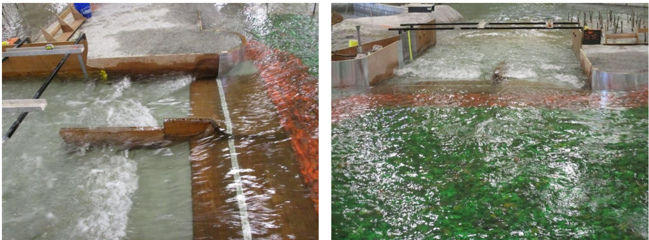
Figure 142. Flow patterns generated in the service spillway with the diversion inlet gates closed at 760 \text{ m}^3/\text{s} .
