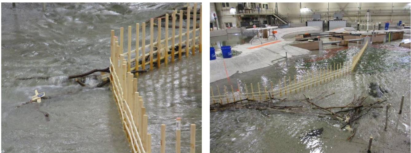
Figure 168. Debris being caught on the barrier and protruding out into the river (left), and this phenomenon continuing to bridge across the river against the standing trees producing a jam (right).
