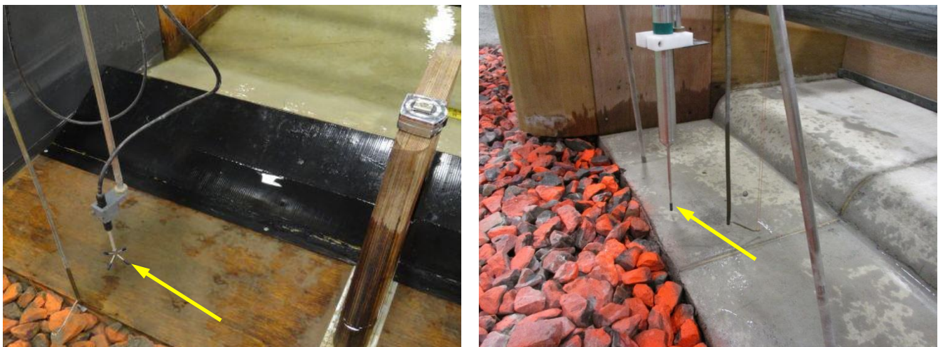
Figure 79. Three-axis acoustic Doppler velocimeter (left) two-axis electromagnetic current meter (right).
