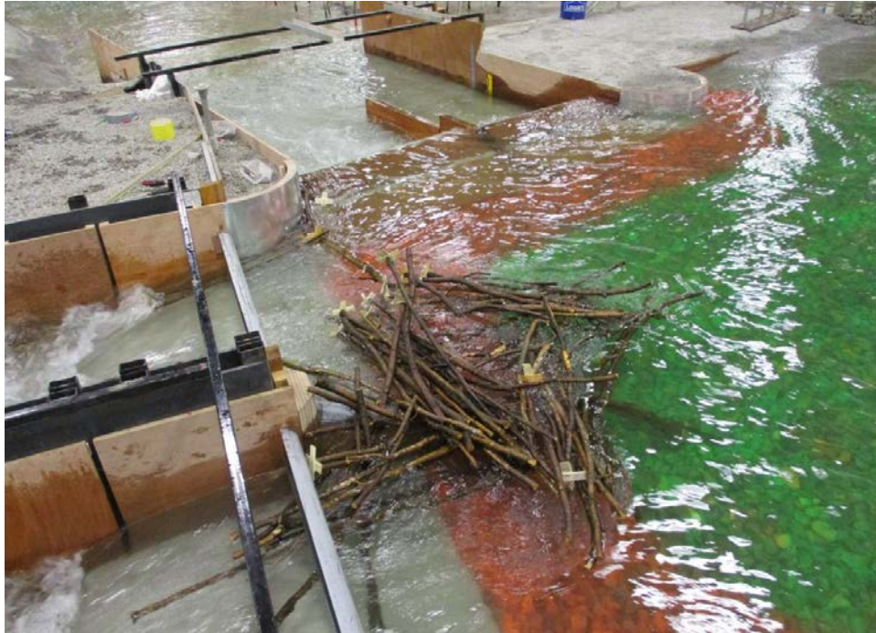
Figure 132. Debris caught on Pier Nose 4.
