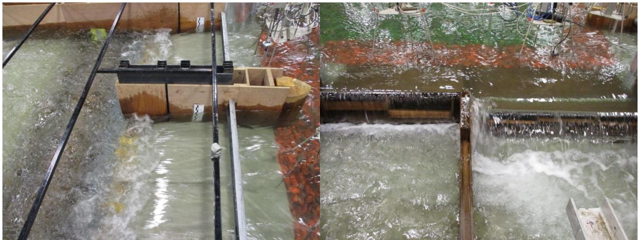
Figure 159. Flow through the diversion inlet structure (left) and service spillway (right) during the 760 m 3 /s case (a) flood condition.
