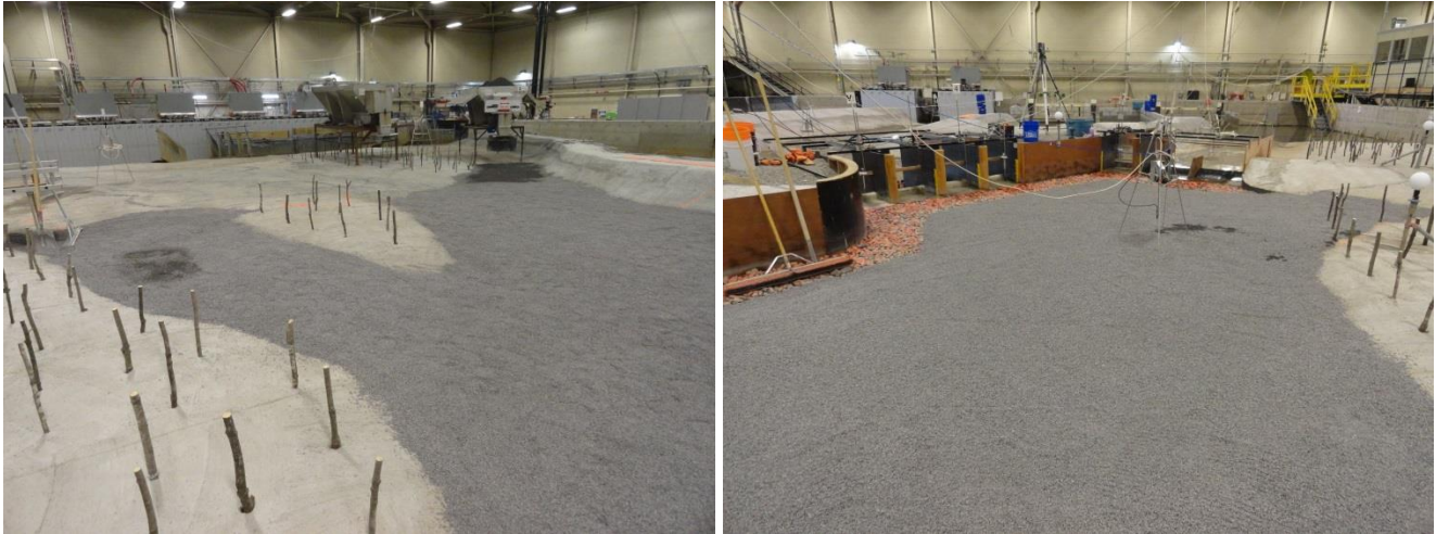
Figure 102. Initial sediment preloading in the upstream (left) and forebay (right) areas.
