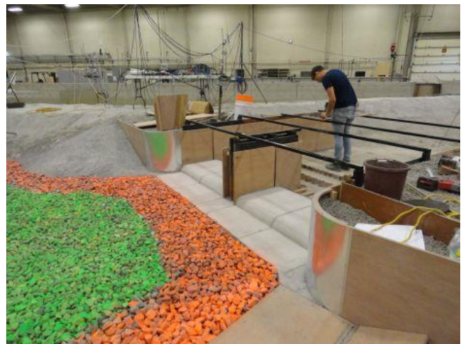
Figure 52. Left: diversion inlet concrete apron and breast wall (the lift gate is closed). Right: installation of the 440kg riprap (orange) and the 210kg riprap stone used to model the mobile-bed portion of the model (green).
