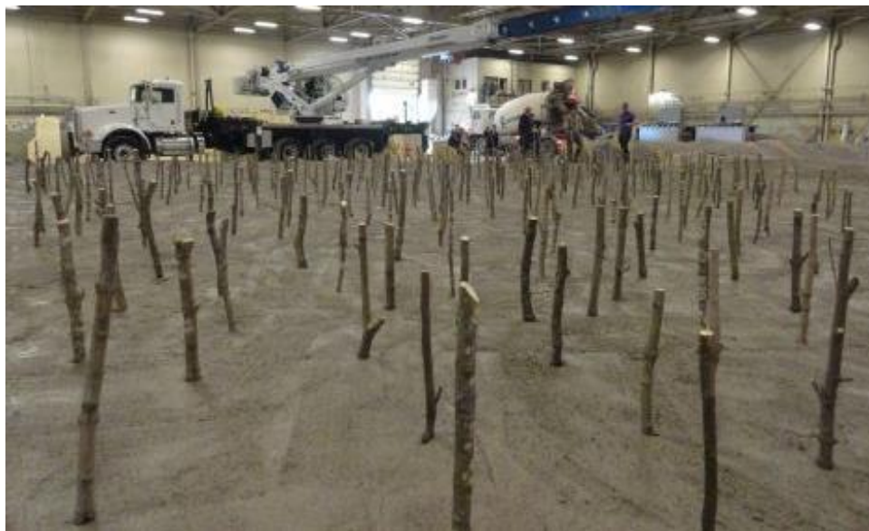
Figure 32. Model trees in the curing concrete.
