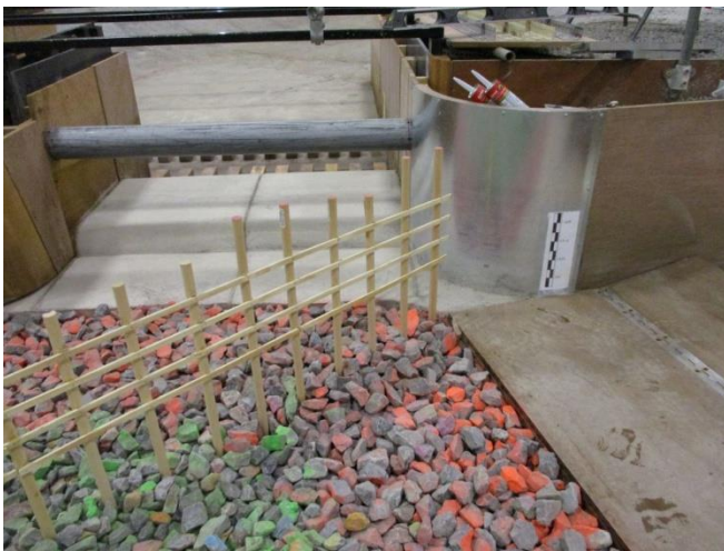
Figure 65. Debris Barrier E implementation in the model.
