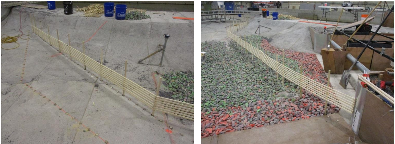
Figure 67. Debris Barrier F construction in the model.
