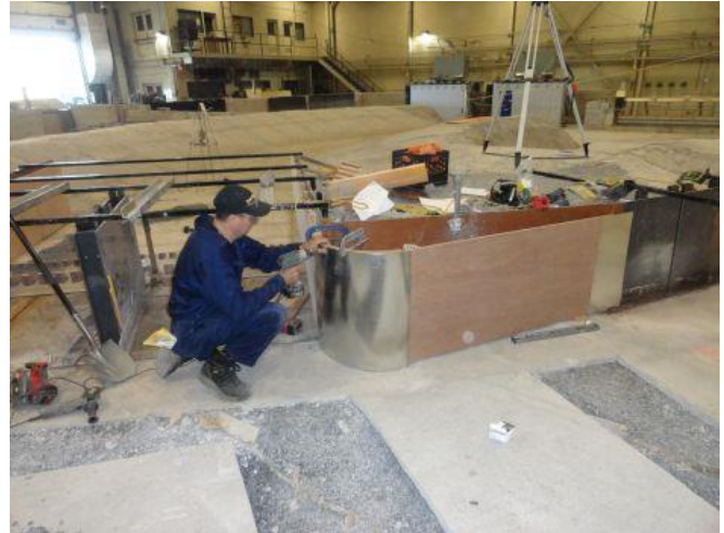
Figure 51. Installing the modified central retaining wall between the diversion inlet and service spillway.
