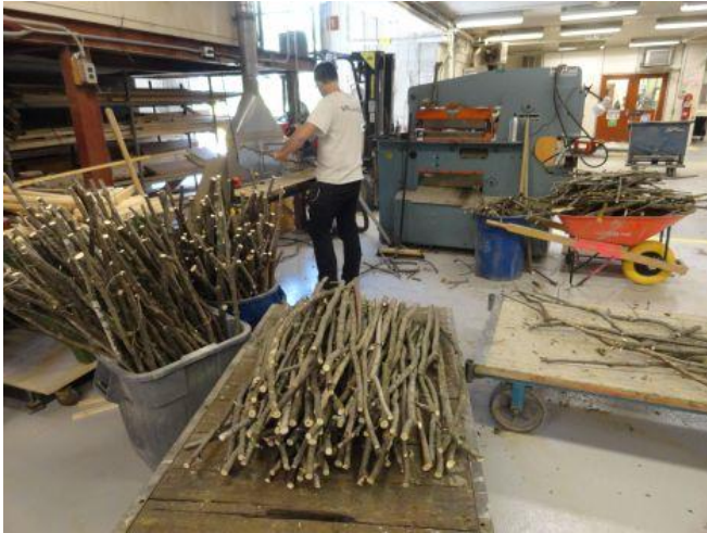
Figure 68. Left - woody debris preparation, right – standing trees cast into the model concrete.
