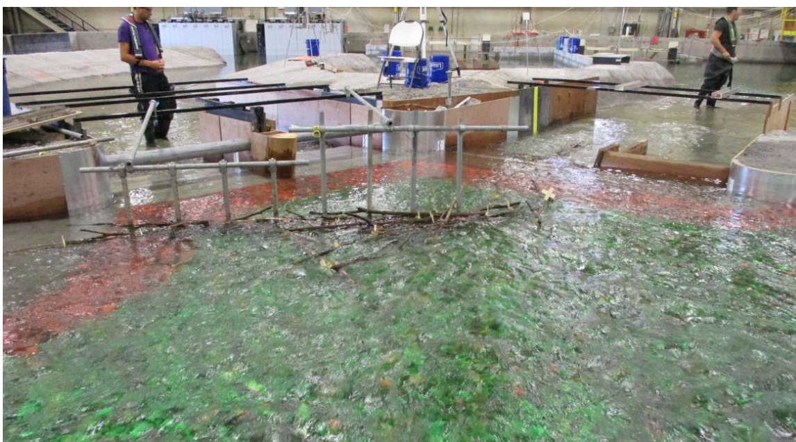
Figure 155. Model trees collecting on debris barrier C during the 320m 3 /s flow.
