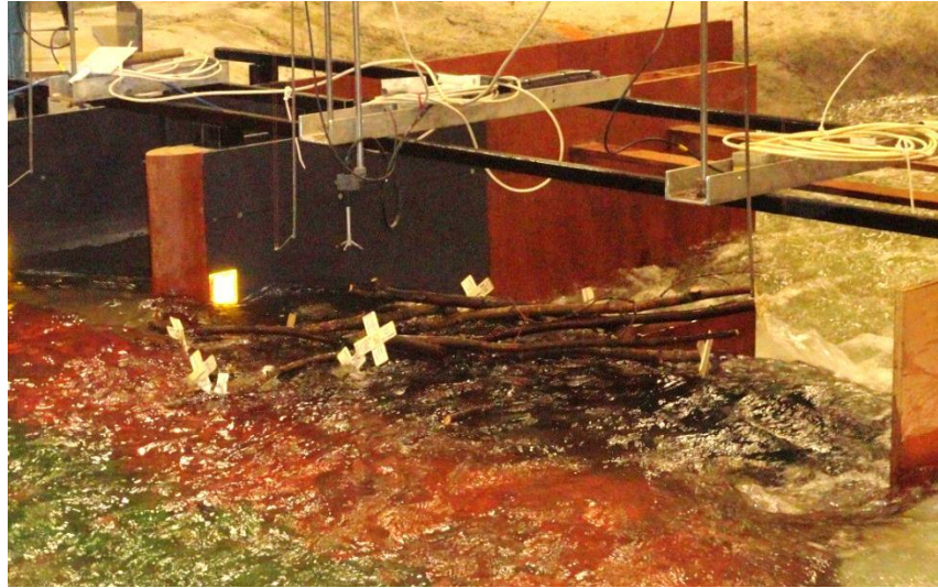
Figure 100. Tree raft snagged on piers in the service spillway.
