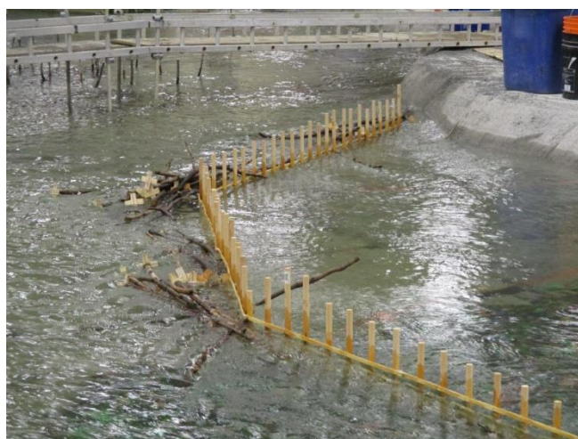
Figure 172. Left - Debris being caught on the barrier and protruding out into the river and this phenomenon continuing to bridge across the river against the standing trees producing a jam. Right – debris trapped in the barrier at the end of the tests.
