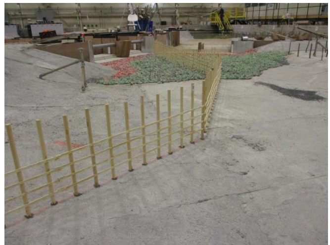
Figure 65. Debris Barrier E implementation in the model.
