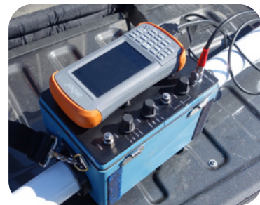
An electromagnetic (EM) induction device. The device emits electromagnetic fields that penetrate the ground to a depth of about five metres. The more mineralized the subsurface water, the higher the electromagnetic conductivity reading. Higher electromagnetic conductivity readings may indicate impacted groundwater. NRCB SciTech staff conduct EM surveys at confined feeding operations to help identify areas of possible groundwater impact.
