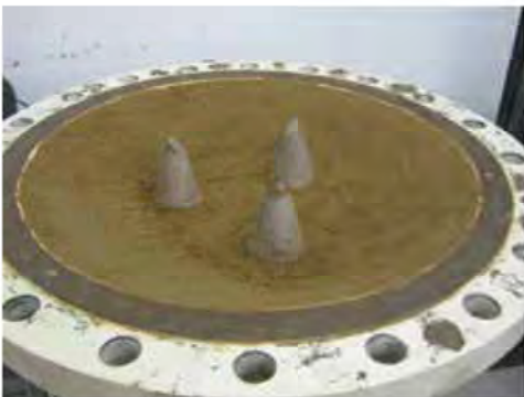
Figure 6. Truncated cones used for testing on subgrade
