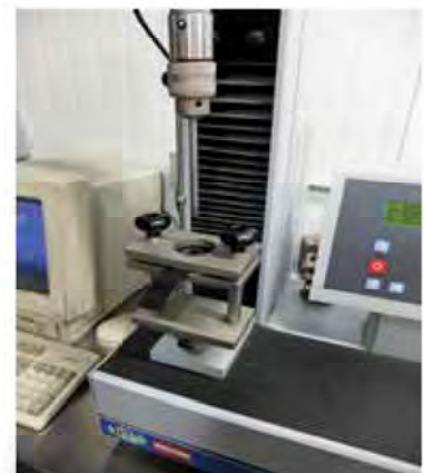
Figure 5. Standard Puncture Test Equipment
