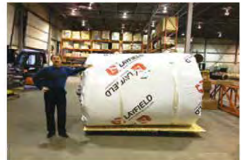
Figure 14. 7000 lbs (3200 ks) one-piece prefabricated Enviro Liner® 6030
