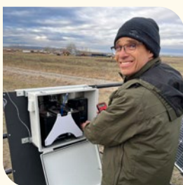
A member of the NRCB SciTech staff checks the voltage of the power supply for an air quality monitoring unit
