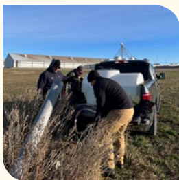
NRCB SciTech and Compliance staff add fluorescent dye to an earthen manure storage
