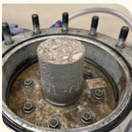
An RCC core undergoing testing in the lab
