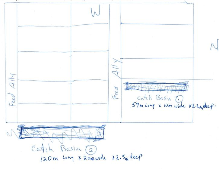
AO note: Two cath basins were constructed with the above dimensions, versus the three proposed and permitted in LA22001
