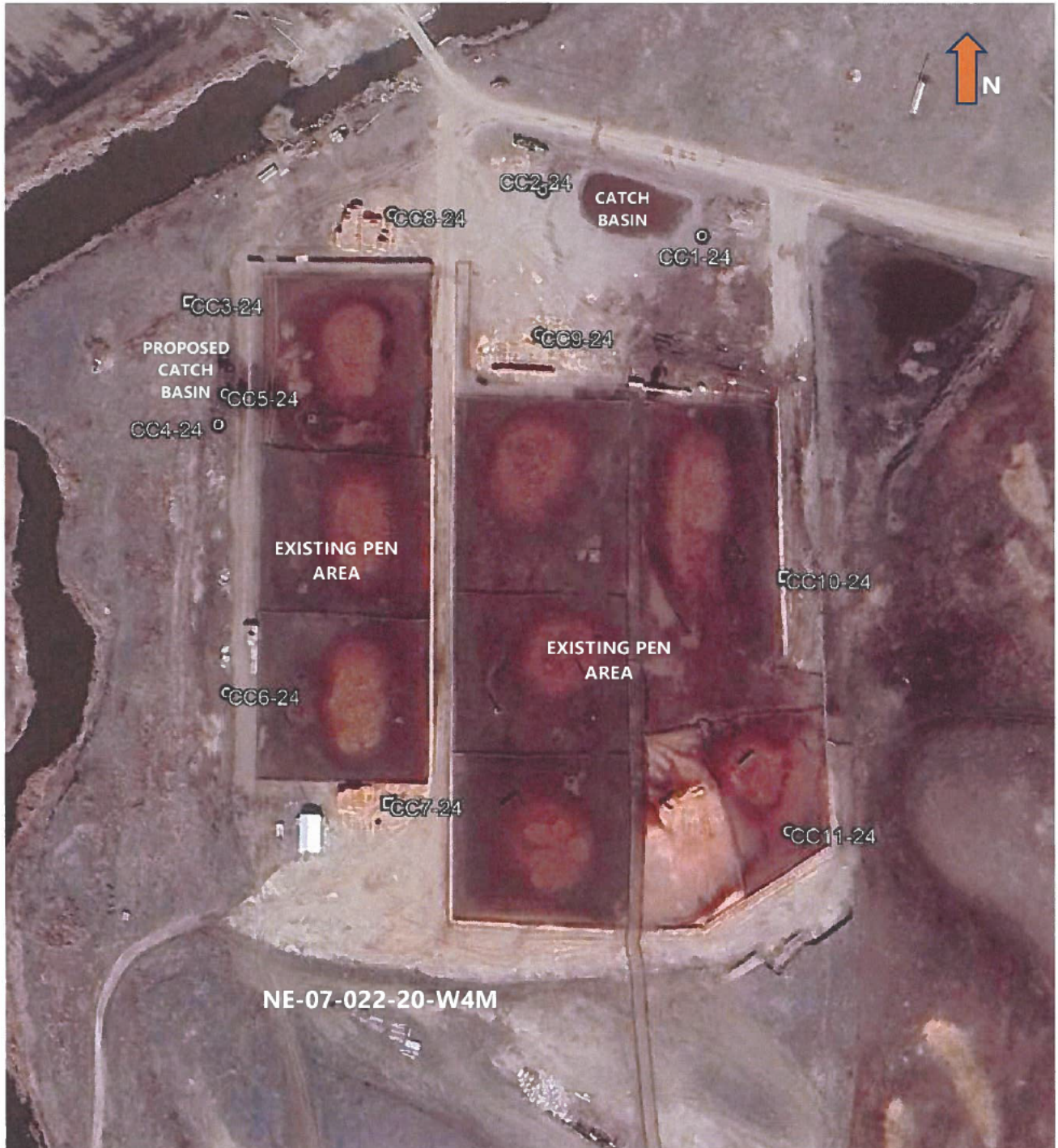
Figure 1: Site Layout & Borehole Locations
